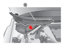
3. Unfasten the 3 clips and remove the cowl top cover (B) by pulling it towards the front of the vehicle.
