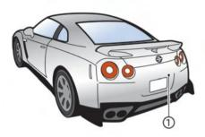
If dirt, rain or snow accumulates on the camera (), the RearView Monitor may not display objects clearly. Clean the camera by wiping it with a cloth dampened with a diluted mild cleaning agent and then wiping it with a dry cloth.
