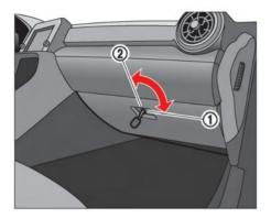
The mechanical key stops when it is inserted approximately halfway in.
