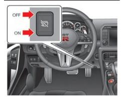
The exhaust sound control switch on the lower side of the instrument panel allows the driver to turn the exhaust sound control system on and off.
