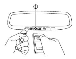
Using both hands, simultaneously press and hold the desired HomeLink® button and handheld transmitter button. DO NOT release until the HomeLink® indicator light ① flashes slowly and then rapidly. When the indicator light flashes rapidly, both buttons may be released. (The rapid flashing indicates successful programming.)
