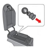
Inside the console box Open the cap to use the outlet. Close the cap after use.
