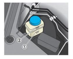
Check the fluid level in the reservoir. If the fluid is below the MIN line ① or the brake warning light comes on, add Genuine NISSAN Brake Fluid R35 Special II fluid (or equivalent) up to the MAX line ②. If fluid must be added frequently, the system should be checked. It is recommended you contact a GT-R certified NISSAN dealer.
