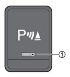
The sonar system OFF switch on the lower side of the instrument panel allows the driver to turn the sonar system on and off. To turn the sonar system on and off, the ignition switch must be in the ON position. The indicator light ① on the switch will turn off when the system is turned off. If the indicator light flashes it may indicate a malfunction in the sonar system.
