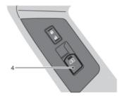
Front passenger's side4. Front passenger's window switch
