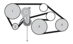
ess. If the belt is in poor condition or loose, have it replaced or adjusted. It is recommended you contact a GT-R certified NISSAN dealer.
