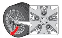
7. Tighten the wheel nuts by hand by turning them clockwise until the tapered part (a) of each nut lightly contacts the seat part (b) of the wheel hole.
