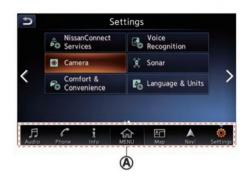
If the RearView Monitor is not in operation, change the setting according to the following procedure.
