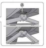
4. Carefully raise the vehicle until the tire clears the ground. To lift the vehicle, securely hold the jack lever and rod with both hands as shown above.
