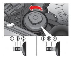
• Adjust the power steering fluid level to the R mark (5) on the power steering dipstick when the fluid temperature is hot or (6) when the fluid temperature is cold.
