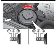
Check the fluid level in the reservoir. Remove the cap that is attached with a gauge inside.
