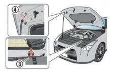
3. Grasp the insulated part of the stay ③ and release it from the hook, then securely insert it into the hood hole ④.
