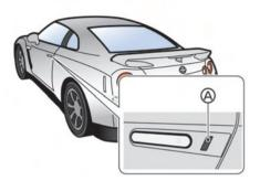
When you carry the Intelligent Key with you, you can lock or unlock all doors by pushing the door handle request switch  $\bigotimes$  within the range of operation.
