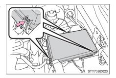
Under the instrument panel Remove the cover.
