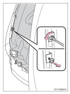
2 Open the fender liner and unplug the connector while depressing the lock release.
