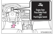
Press the engine switch shortly and firmly.
