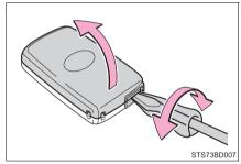
3 Remove the depleted battery.
