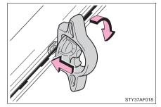
3 Slide the cleat to the closest detent in the rail system. You will feel that the locking plate snaps into a detent.
