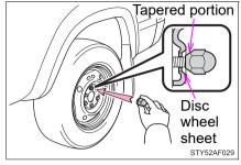
▶ Replacing an aluminum wheel with a spare steel wheel
