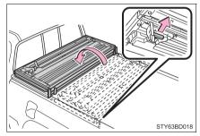
4 Secure by using the storage straps.
