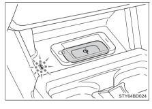
When placing the mobile device on the wireless charging surface of the tray, make sure that there are no objects in-between the mobile device and the tray. They may interfere with charging.
