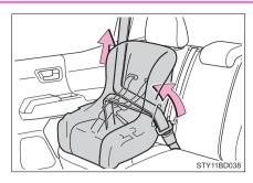
5 If the child restraint has a top tether strap, the top tether strap should be latched onto the top tether strap anchor. (→P. 66, 68)
