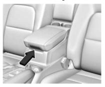
There is storage under the armrest in the center console. Press the button and lift.
