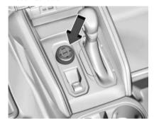
To activate each mode, turn the MODE knob on the center console in either direction.
