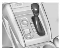
The electronic shift lever position indicator, next to the shifter, comes on when the vehicle is on or in accessory mode. There is also a gear position indicator in the Driver Information Center.
