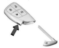
Press the button on the side of the remote key near the bottom and pull the mechanical key out. Never pull the mechanical key out without pressing the button.
