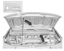
Lift the hood only enough to release the hood prop rod from its retainer, and insert it into the slot marked with an arrow on the underside of the hood. Lifting the hood too far may disengage the parts adjacent to the hinges.
