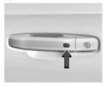
If equipped, the remote key must be within 1 m (3 ft) of the tailgate or door being opened or locked. Press the button on the door handle to open. See "Keyless Access Operation" in Remote Key Operation ▷ 8.
