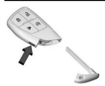
Remove the key by pressing the button on the side of the remote key near the bottom and pull the key out. Never pull the key out without pressing the button.
