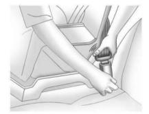
Push the latch plate into the buckle until it clicks. Position the release pushbutton on the buckle, away from the child restraint, so that the seat belt could be quickly unbuckled if necessary.
