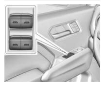
Power windows work when the vehicle is on, in accessory mode, or when Retained Accessory Power (RAP) is active. See *Retained Accessory Power (RAP)* ⇒ 170.
