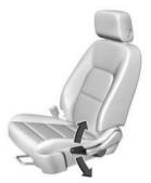
If equipped, move the lever up or down to raise or lower the seat.
