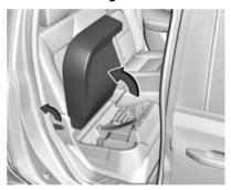
If equipped, there is storage under the rear seat. Pull the release lever and then raise the seat cushion. Pull the lever again to lower the cushion.
