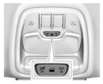
The dome lamps and dome lamp controls are in the overhead console.
