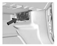
There is a cover on the instrument panel fuse block. Press the clips on the side to remove the cover.
