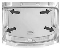
The vehicle may be equipped with four cargo tie-downs in the rear compartment.
