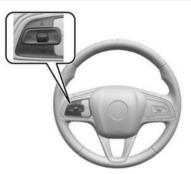
S: Press to turn cruise control on and off. A white indicator light appears in the instrument cluster when cruise control is turned on.
