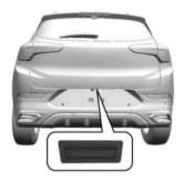
To open the liftgate, press the touch pad under the liftgate handle and lift up.
