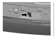
2. Go to the front of the vehicle and move the secondary hood release lever toward the right side of the vehicle.
