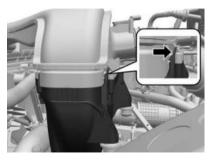
3. Disassemble the duct.
