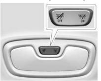
If equipped, the rear dome light switch are in the headliner above the rear seats.
