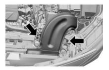
1. Remove the two push pins.
