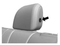
To fold the head restraint, press the button on the side of the head restraint.
