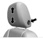
To raise or lower the head restraint, press the button located on the side of the head restraint, and pull up or push the head restraint down, and release the button. After releasing the button, ensure the head restraint locks in place and is unable to move up or down.
