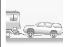
To tow a front-wheel-drive vehicle from the front with two wheels on the ground:
