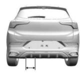
To operate, move your foot in a forward kicking motion near the left side of the rear bumper at the location of the projected logo, then pull it back. The kick must come within 14 cm (6 in) of the rear bumper to activate. Then step back.
