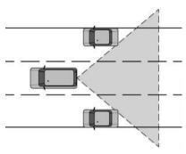
If equipped, this automatic dimming mirror provides a wide angle camera view of the area behind the vehicle.
