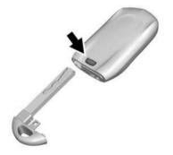
To remove the key, press the button on the bottom of the remote key and pull the key out. Never pull the key out without pressing the button.
