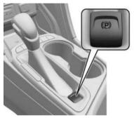
The Electric Parking Brake (EPB) can always be applied, even if the vehicle is off. In case of insufficient electrical power, the EPB cannot be applied or released. To prevent draining the battery, avoid unnecessary repeated cycles of the EPB.
