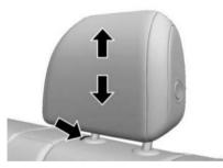
To lower the head restraint, press the button located on the top of the seatback and push the head restraint down. After releasing the button, ensure the head restraint locks in place and is unable to move up or down.
