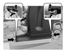
2. Press a hook both sides and disassemble two hooks.
