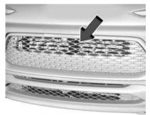
This vehicle may have a shutter system that automatically closes the frontal cooling opening. This system is designed to help improve fuel economy. Ensure the shutter system is clear of any visible debris, snow, or ice.
