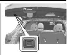
Press any liftgate button, the touch pad, or  $\frac{2}{3}$  on the remote key while the liftgate is moving to stop it. Pressing any liftgate button or pressing  $\frac{2}{3}$  twice quickly on the remote key restarts the operation in the reverse direction. Pressing the touch pad on the liftgate handle will restart the motion, but only in the opening direction.
