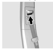
To move the shoulder belt height adjuster down, push up on the release button and move the height adjuster to the desired position. You can move the height adjuster up by pushing up on the shoulder belt guide.
