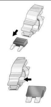
3. Use the fuse puller to remove the fuse from the top or side, as shown above.
