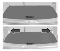
The cargo management system has a height adjustment. Place the load floor on the holders.
