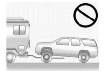
All-wheel-drive vehicles must not be towed with two wheels on the ground.
