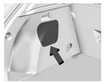
The rear compartment fuse block is behind a cover on the driver side of the rear compartment. To access the fuses, remove the cover.
