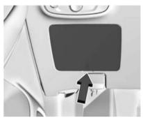
The instrument panel fuse block is on the underside of the driver side instrument panel. To access the fuses, open the fuse cover by pulling out. To reinstall the cover, insert the top tab first, then push the cover back into its original location.
