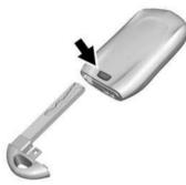
Press the button on the bottom of the remote key to remove the key. Never pull the key out without pressing the button.
