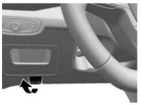
1. Pull the hood release handle inside the vehicle. It is located on the lower left side of the instrument panel.
