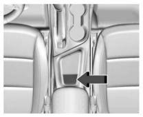
3. Remove the two recognized remote keys from remote key pocket. Place the new remote key in remote key pocket.
