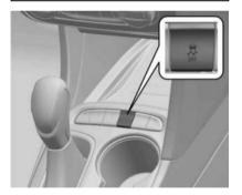
To turn off the Traction Control System, press and release  $\frac{1}{24}$ . The Traction Off light (2) displays in the instrument cluster. To turn the Traction Control System on again, press and release  $\frac{1}{24}$ . See *Traction Off Light*  $\stackrel{1}{\sim}$  108.
