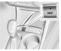
Press the AWD button on the center console to activate the system. The indicator light flashes briefly while the system engages and stays lit when the AWD system is active. See All-Wheel-Drive Light  $\Rightarrow$  107.
