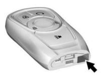
2. Insert a flat, thin object and remove the back cover.
