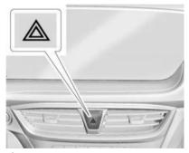
A: Press to make the front and rear turn signal lights flash on and off. This warns others that you are having trouble.
