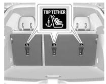
The top tether anchors for each rear seating position are on the back of the rear seatback. For models with a cargo cover, remove the cargo cover before installing the top tether. The cargo cover should remain off while the top tether is in use. Be sure to use an anchor on the same side of the vehicle as the seating position where the child restraint will be placed.
