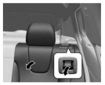
3. Pull the lever on top of the seatback to unlock the seatback.
