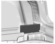
The quarter lower storage panel can be removed on the passenger side. Lift the load floor to access and pull the panel to remove.
