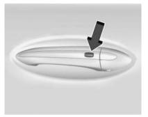
The remote key must be within 1 m (3 ft) of the liftgate or door being opened. Press the button on the door handle to open. See *Remote Key Operation*  $\Leftrightarrow$  9.
