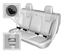
The lower anchors are behind the vertical openings in the seat cushion trim located below the anchor label.
