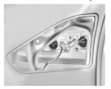
2. Remove the bulb from the bulb socket and replace with a new bulb.
