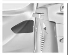
1. Remove the bulb access door on liftgate.
