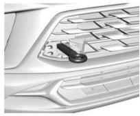
Carefully open the cover on the fascia by using the small notch that conceals the tow eye socket.
