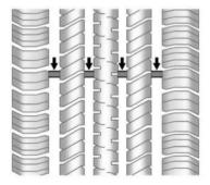
Treadwear indicators are one way to tell when it is time for new tires. Treadwear indicators appear when the tires have only 1.6 mm (1/16 in) or less of tread remaining. See *Tire Inspection*  $\Rightarrow$  254 and *Tire Rotation*  $\Rightarrow$  254.
