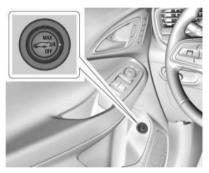
If equipped, the power liftgate switch is on the driver door. The vehicle must be in P (Park).
