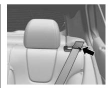
2. Make sure the seat belt is in the retainer hook
