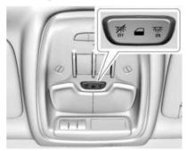
The front dome lights provide overhead interior lighting. The dome light switch is in the overhead console and has three positions.
