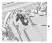
3. Loosen the negative battery cable nut (1).
