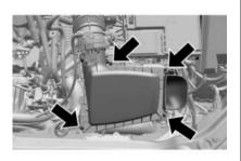
4. Remove four screws, tilt the cover, and slide it out of the assembly.
