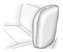
On vehicles with second row seat-mounted side impact airbags, they are in the sides of the seatback closest to the door.
