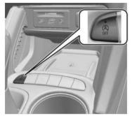
The automatic engine Stop/Start feature can be disabled and enabled by pressing (A). Stop/ Start is enabled each time you start the vehicle.
