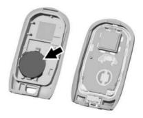
3. Lift the battery with a flat object.
