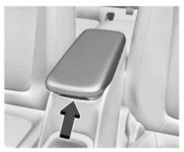
The center console has storage under the armrest. Push the latch and lift the armrest to open. There may be a small storage bin inside. Remove the small bin to access more storage.
