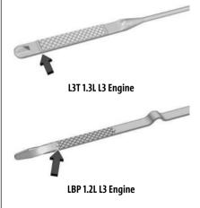
If the oil is below the cross-hatched area at the tip of the dipstick and the engine has been off for at least 15 minutes, add 1 L (1 qt) of the recommended oil and then recheck the level. See "Selecting the Right Engine Oil" later in this section for an explanation of what kind of oil to use. For engine oil crankcase capacity, see *Capacities and Specifications* \$ 296.
