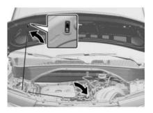
Lift the hood and release the hood prop from its retainer, above the radiator. Securely place the hood prop into the slot on the underside of the hood.
