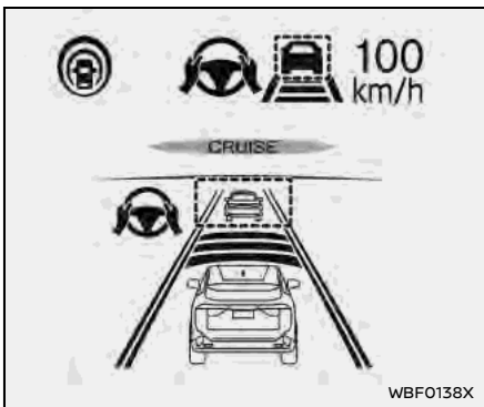
System set display – a vehicle detected ahead (for ProPILOT Assist with Navi-link)
