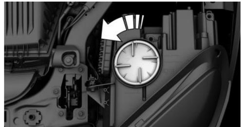
3. Tilt the bulb holder up, arrow 1, and pull it out of the headlight toward the rear, arrow 2.
