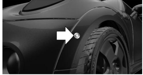
The ultrasound sensors for measuring parking spaces are located on the wheel housing.
