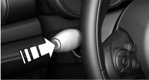
Press and hold button on signal lever.
