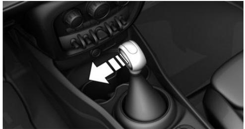
Press the selector lever to the left out of selector lever position D.
