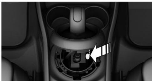
4. Press the button on the front of the selector lever and move the selector lever back slightly.
