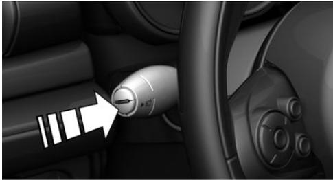
Position of switch, depending on the vehicle equipment:
