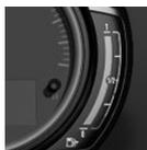
The arrow beside the fuel pump symbol shows which side of the vehicle the fuel filler flap is on.
