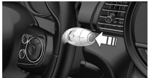
Press the button on the wiper lever.
