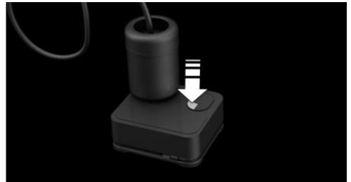
Let the compressor run for max. 10 minutes to fill the tire with sealant and achieve a tire inflation pressure of approx. 2.5 bar. While the tire is being filled with sealant, the tire inflation pressure may sporadically reach approx. 5 bar. Do not switch off the compressor at this point.
