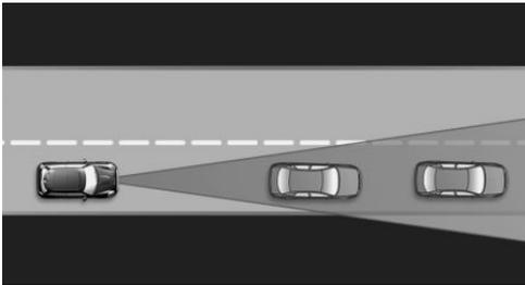
The detection capacity of the system and the automatic braking capacity are limited. Two-wheeled vehicles for instance might not be detected.
