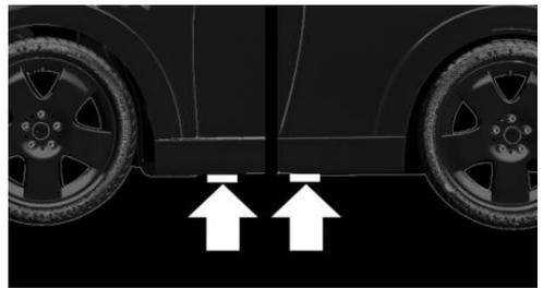
The jacking points for the vehicle jack are located at the marked positions.
