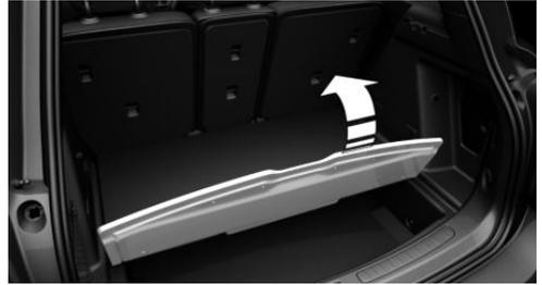
2. Place the MINI Picnic Bench on the front part of the cargo floor panel and attach it to the rear part of the cargo floor panel using the four snaps.
