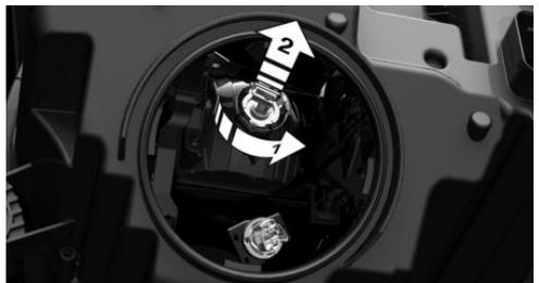
5. Pull the bulb out of the bulb holder.
