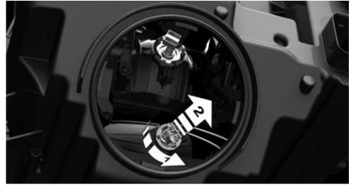
5. Press the bulb gently into the bulb holder, turn counterclockwise and remove.
