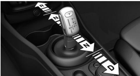
The selector lever positions P, R, N, and D are selected by tapping the selector lever
