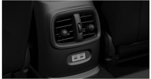
One USB dual charge socket is located in the rear center console.
