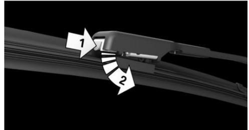
4. Attach a new wiper blade. The wiper blade must engage audibly.
