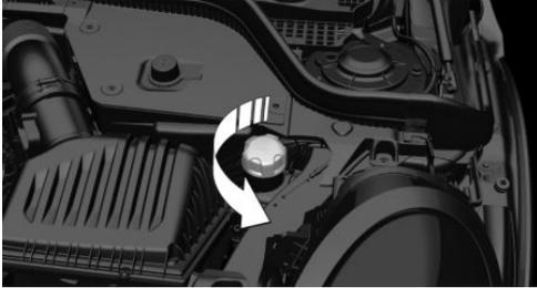
4. If the coolant is low, slowly add coolant up to the specified level; do not overfill.
