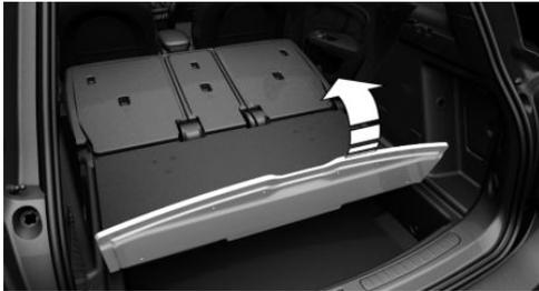
3. Grasp the cargo floor panel in the rear and fold up above the locking point of the upper position, refer to page 233.
