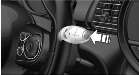
Press the button on the wiper lever.
