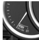
The display indicates that the Auto Start/Stop function is ready for an Automatic engine start.
