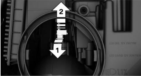
4. Pull the bulb out of the bulb holder.
