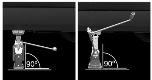
7. Crank up the vehicle jack until the entire surface of the jack is in contact with the ground and the wheel in question is
