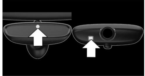
Photocells are used for control:
