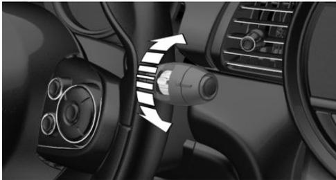
Turn the thumbwheel on the wiper lever.
