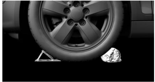
Place wheel chocks or other suitable objects in front and behind the wheel that is diagonal to the wheel to be changed.
