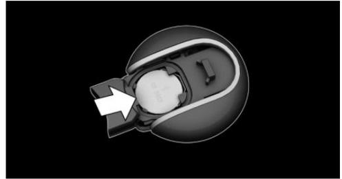
5. Insert a type CR 2032 battery with the positive side facing up.
