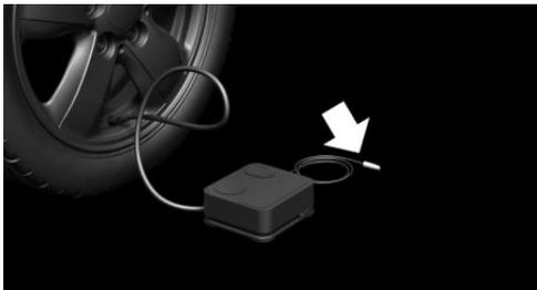
5. With the ignition switched on or the engine running, switch on the compressor.
