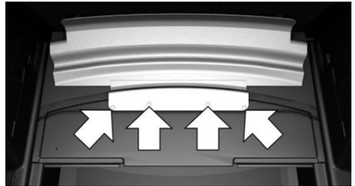
3. Fold down the MINI Picnic Bench toward the rear. The MINI Picnic Bench is fastened with magnets.
