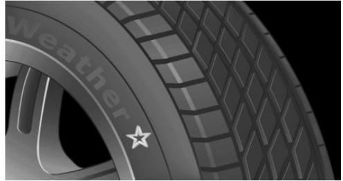
For each tire size, the manufacturer of the vehicle recommends certain tire brands. The tire brands can be identified by a star on the tire sidewall.
