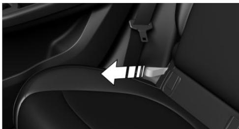
2. Fold the rear seat backrest rearward. The rear seat backrest first engages in the loading position.
