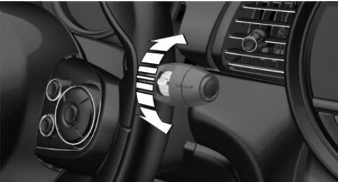
Turn the thumbwheel on the wiper lever.
