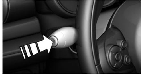
Press and hold button on signal lever.
