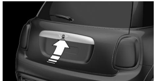
Unlock the vehicle and press the button on the tailgate.
