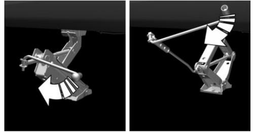
4. Take your hand away from the vehicle jack as soon as the vehicle jack is under load and continue turning the vehicle jack crank or lever with one hand.
