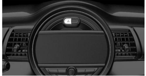
The button is located above the Control Display.
