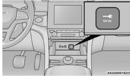
Front Power Outlet
