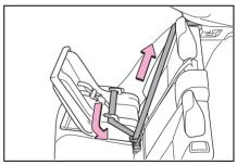
6 After installing the child restraint system, rock it back and forth to ensure that it is installed securely. (→P.59)
