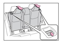
2 Pull the head restraint up while pressing the lock release button A.
