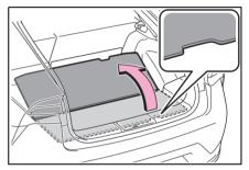
2 Hold the handle and pull it toward you, and then the 3 clips will be disengaged
