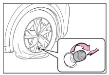
6 Extend the hose. Remove the air release cap from the hose.
