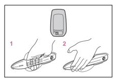
1 Grip the driver's door handle to unlock the door. Holding the driver's door handle for approximately 2 seconds unlocks all the doors. Grip the front passenger's door handle with the sensor (if equipped) to unlock all the doors.\*
