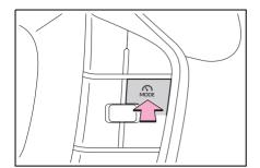
2 Using the accelerator pedal, accelerate or decelerate to the desired vehicle speed (approximately 20 mph [30 km/h] or more), and press the driving assist switch to set the set vehicle speed.
