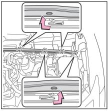
Disconnect the claws and remove the service cover.
