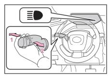
With the headlights on, push the lever away from you to turn on the high beams. Pull the lever toward vou to the center position to turn the high beams off.
