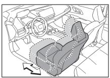
When all of the following have been performed, the driver's seat is automatically adjusted to a position that allows driver to enter and exit the vehicle easily.
