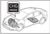
Electricity generated by the gasoline engine can be used to charge the hybrid battery (traction battery) by switching to the hybrid battery (traction battery) charge mode when electricity needed for EV driving is not remaining.\*
