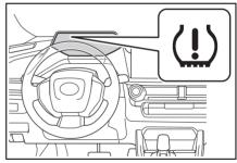
9 If the specified tire inflation pressure of the wheel set installed differs from that of the previous set, it will be necessary to perform the tire inflation pressure setting procedure of the tire pressure warning system. (→P.520)
