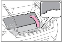
Hold the handle and pull it toward you, and then the 3 clips will be disengaged
