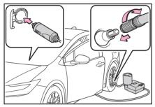
21Turn the compressor switch on and wait for several seconds, then turn it off. Check the tire inflation pressure.
