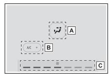
A Select the air flow mode Each time the switch is touched, the air flow mode changes.
