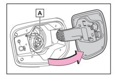
4 Remove the charging connector cap and secure it to the cable.
