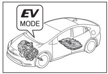
When a sufficient amount of electricity is remaining after charging\*1, EV driving is performed using electricity stored in the hybrid battery (traction battery).\*2
