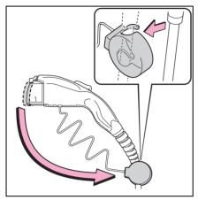
5 Insert the charging connector into the AC charging inlet.
