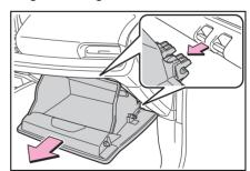
5 Unlock the filter cover (A), pull the filter cover out of the
