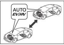
Normally, the electricity stored in the hybrid battery (traction battery) is used for EV driving. However, when more power is required, such as for driving uphill or accelerating suddenly, the gasoline engine starts and provides powerful acceleration by strongly depressing the accelerator pedal.
