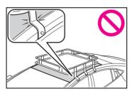
Do not load luggage directly onto the solar roof.
