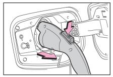
3 Attach the charging connector cap.
