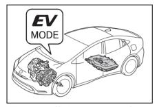
When a sufficient amount of electricity is remaining after charging\*1, EV driving is performed using electricity stored in the hybrid battery (traction batterv).\*2
