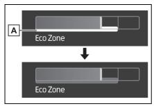
The engine braking force will be increased according to the driving conditions to more efficiently charge the hybrid battery (traction battery) after the accelerator pedal is released.
