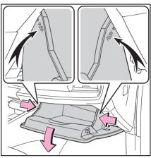
With the glove box fully open, slightly lift up the glove box and pull toward the seat to detach the bottom of the glove box.
