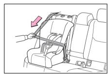
6 While pushing the child restraint system into the rear seat, allow the shoulder belt to retract until the child restraint system is securely in place.
