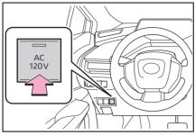
3 Open the lid, and fully and securely insert the plug of the device into the power outlet. (→P.473)
