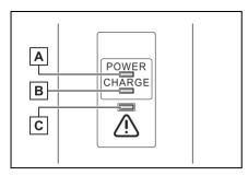
A Power indicator Illuminates when electricity is flow-
