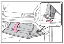
3 Push in each side of the glove box to disconnect the claws, and then slowly and fully open the glove box while supporting it.
