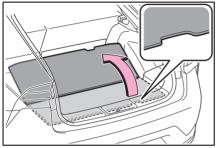
2 Raise the hook to use, return the deck board to its original position and close it.
