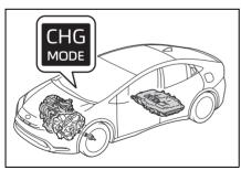
Electricity generated by the gasoline engine can be used to charge the hybrid battery (traction battery) by switching to the hybrid battery (traction battery) charge mode when electricity needed for EV driving is not remaining.\*
