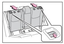
2 Align the head restraint with the installation holes and push it down to the lowest lock position.
