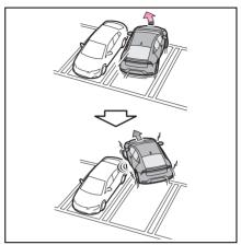
■ When reversing and a collision with a stationary object on the outer side of a turn is likely
