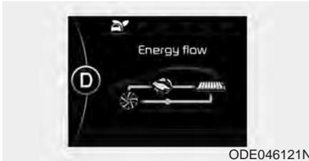
Hybrid battery is being charged by regenerative braking.
