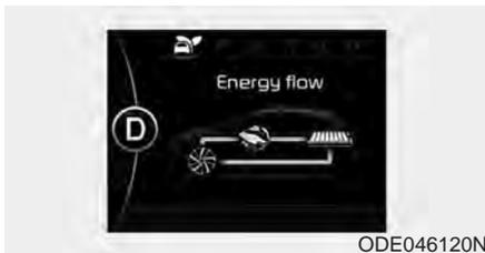
The mode means the vehicle is at a complete stop. (There is no energy flow.)
