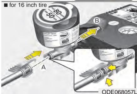
2. Connect the filling hose (3) onto the connector of the sealant bottle (A).
