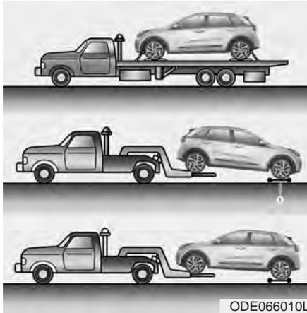
On FWD vehicles, it is acceptable to tow the vehicle with the rear wheels on the ground (without dollies) and the front wheels off the ground. If any of the loaded wheels or suspension components are damaged or the vehicle is being towed with the front wheels on the ground, use a towing dolly under the front wheels. When being towed by a commercial tow truck and wheel dollies are not used, the front of the vehicle should always be lifted, not the rear.
