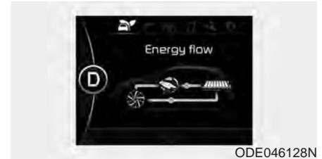
The engine and regenerative braking system is charging the hybrid battery through deceleration.
