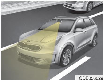
The Lane Keeping Assist System detects the lane markers on the road with a front view camera at the front windshield, and assists the driver's steering to help keep the vehicle in the lanes.
