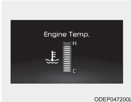
This gauge indicates the temperature of the engine coolant when the engine is running.
