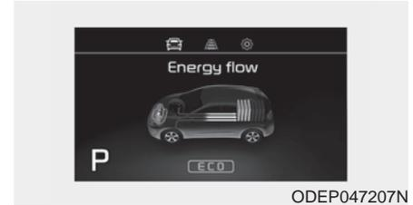
The engine and regenerative braking system charge the hybrid battery driving deceleration.
