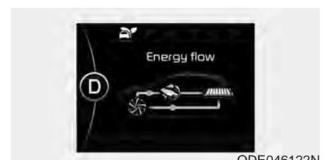
The engine compression can be used to slow the vehicle. The regenerative braking system can be used to charge the hybrid system.
