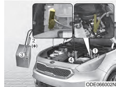
Connect cables in numerical order and disconnect in reverse order.
