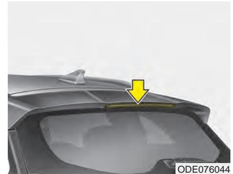
If the high mounted stop lamp (LED) does not operate, have the vehicle checked by an authorized Kia dealer.
