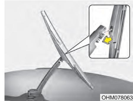
2. Install the new blade assembly by inserting the center part into the slot in the wiper arm until it clicks into place.
