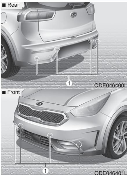
The parking assist system assists the driver during movement of the vehicle by chiming if any object is sensed within the distance of 39 in. (100 cm) in front and 47 in. (120 cm) behind the vehicle.
