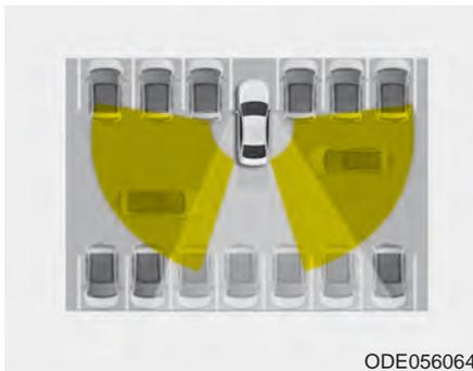
When your vehicle moves in reverse from a parking position, the sensor monitors approaching vehicles to the left and right side of the vehicle and gives information to the driver.
