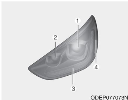
If the Low/High beam lamp (1), Low beam lamp (2), Front turn signal lamp/Position lamp(3), or side marker (4) does not operate, have the vehicle checked by an authorized Kia dealer.
