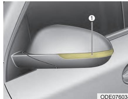
If the side repeater lamp (LED) does not operate, have the vehicle checked by an authorized Kia dealer. The LED lamps cannot be replaced as a single component because they are part of an integrated unit. The LED lamps has to be replaced with the unit.
