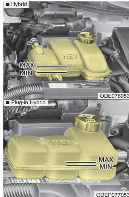
The coolant level should be filled between MAX and MIN marks on the side of the coolant reservoir when the engine is cool.
