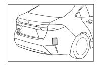
Do not attach accessories, stickers (including transparent stickers), aluminum tape, etc. to a sensor or its surrounding area on the rear bumper. 4
