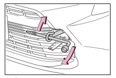
5 Securely attach cables or chains to the towing eyelet.
