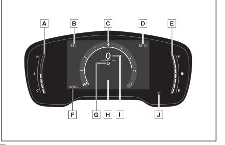
A Engine coolant temperature gauge
