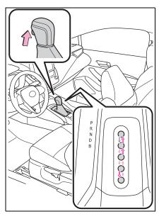
While the engine switch is in ON and the brake pedal depressed<sup>\*</sup>, shift the shift lever while pushing the shift release button on the shift knob.
