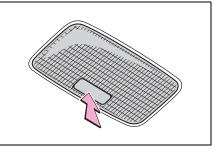
Turns the lights on/off When the door position is on for the front interior lights, the rear interior light will turn on when a door is open and turn off when all of them are closed.
