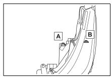
A Adjustment bolt A B Adjustment bolt B
