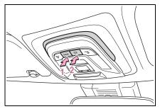
1 Turns the door position on/off When a door is opened while the door position is on, the lights turn
