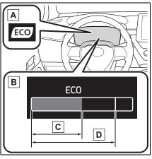
A Eco Driving Indicator Light During Eco-friendly acceleration (Eco driving), the Eco Driving Indicator Light will turn on. When the acceleration exceeds the Zone of Eco driving, or when the vehicle is stopped, the light turns off.
