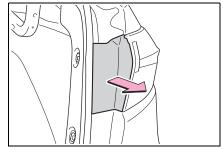
4 Remove the 2 screws and then remove the light assembly by pulling it straight back.
