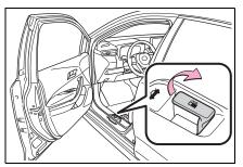
2 Turn the fuel tank cap slowly and remove it, then hang it on the back of the fuel filler door.
