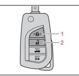
1 Locks all the doors Check that the door is securely locked.
