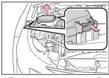
Engine compartment: type B fuse box
