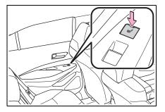
The heated steering wheel and seat heaters can be used when The engine switch is in ON.
