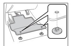
2 Turn the upper knob of each retaining hook (clip) to secure the floor mats in place.
