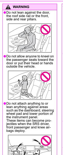
Do not attach anything to areas such as a door, windshield, side windows, front or rear pillar, roof side rail and assist grip.
