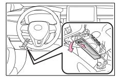
3 Remove the fuse with the pullout tool.Only type A fuse can be removed using the pullout tool.
