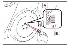
When replacing an aluminum wheel with a steel wheel (including a compact spare tire), tighten the wheel nuts until the tapered portion [A] comes into loose contact with the
