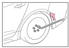
4 Turn the tire jack portion A by hand until the center of the recessed portion of the jack
