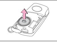
3 Remove the depleted battery using a small flathead screwdriver.
