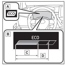
A Eco Driving Indicator Light During Eco-friendly acceleration (Eco driving), the Eco Driving Indicator Light will turn on. When the acceleration exceeds the Zone of Eco driving, or when the vehicle is stopped, the light turns off.
