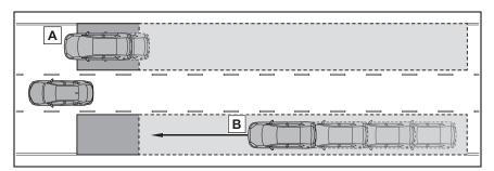
A Vehicles that are traveling in areas that are not visible using the outside rear view mirrors (the blind spots)
