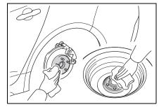
2 Install the tire and loosely tighten each wheel nut by hand by approximately the same amount.
