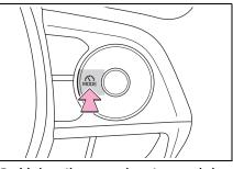
2 Using the accelerator pedal, accelerate or decelerate to the desired vehicle speed (approximately 20 mph [30 km/h] or more), and press the driving assist switch to set the set vehicle speed.
