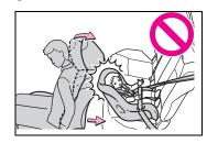
Adjust the front passenger seat so that it does not interfere with the child restraint system.
