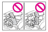
Do not allow a child to stand in front of the SRS front passenger airbag unit or sit on the knees of a front passenger.
