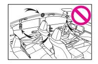
Vehicles without a smart key system: Do not attach any heavy, sharp or hard objects such as keys and accessories to the key. The objects may restrict the SRS knee airbag inflation or be thrust into the driver's seat area by the force of the deploying airbag, thus causing a danger.
