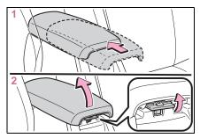
1 Slide the lid to the rear most position. (vehicles with a slide function)
