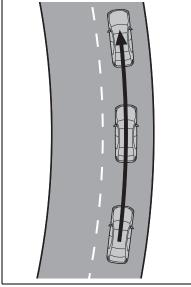
When the function is operating, if the vehicle is likely to depart from its lane, the driver will be alerted via a display and buzzer.
