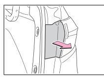
4 Remove the 2 screws and then remove the light assembly by pulling it straight back.
