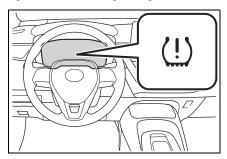
9 If the specified tire inflation pressure of the wheel set installed differs from that of the previous set, it will be necessary to perform the tire inflation pressure setting procedure of the tire pressure warning system. (→P.318)
