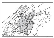
6 Start the engine and turn the air conditioning system on to check that the radiator cooling fan operates and to check for coolant leaks from the radiator or hoses.
