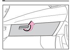
Pull up the lever to open the glove box.
