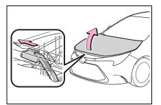
**3** Hold the hood open by inserting the support rod into the slot.
