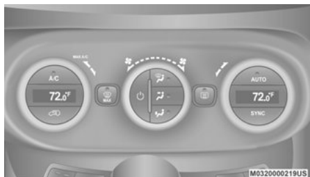
Automatic Climate Controls
