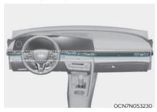
The lamp turns on when **Setup > Vehicle** > **Lights > Ambient Lighting** is selected from the infotainment system.
