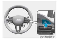
Press the Driving Assist ((\*\*)) button to turn Manual Speed Limit Assist off. The Manual Speed Limit Assist ((\*\*)\*LIMIT) indicator will go off.
