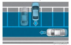
Rear Cross-Traffic Collision-Avoidance Assist may detect vehicles passing by behind you when parking in reverse into a parking space. If this occurs, the function may unnecessarily warn the driver and control the brake.
