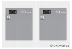
If the speed limit of the road changes during the operation of Manual Speed Limit Assist an arrow in the direction of up or down is displayed to inform the driver that the set speed needs to be changed. At this time, the driver can change the set speed according to the speed limit by using the + or - switch on the steering wheel.
