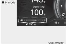
This gauge indicates the approximate amount of fuel remaining in the fuel tank.
