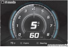
When engine is operating in a high RPM area, it is indicated on the cluster according to the corresponding engine RPM.
