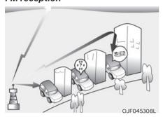
AM and FM radio signals are broadcast from transmitter towers located around your city. They are intercepted by the radio antenna on your vehicle. This signal is then received by the radio and sent to your vehicle speakers.
