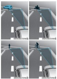
Forward Collision-Avoidance Assist may not detect other vehicles, powered two-wheelers, pedestrians or cyclists in front of you on curved roads that adversely affect the performance of the sensors. This may result in no warning or braking assist when necessary.
