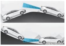
Blind-Spot Collision-Avoidance Assist may not operate properly when driving on a slope. Blind-Spot Collision-Avoidance Assist may not detect the vehicle in the next lane or may incorrectly detect the ground or structure.
