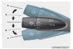
To signal a turn, push down on the lever for a left turn or up for a right turn in position (A). To signal a lane change, move the turn signal lever slightly and hold it in position (B). The lever will return to the OFF position when released or when the turn is completed.
