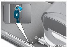
The fuel filler door must be opened from inside the vehicle by pulling up the fuel filler door opener.
