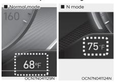
This gauge indicates the current outside air temperatures either in Celsius (°C) or Fahrenheit.
