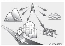
FM broadcasts are transmitted at high frequencies and do not bend to follow the earth's surface. Because of this, FM broadcasts generally begin to fade at short distances from the station. Also, FM signals are easily affected by buildings, mountains, or other obstructions.
