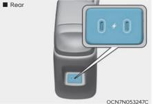
The USB charger is located inside the console box between the driver's seat and the front passenger's seat. Insert the USB charger into the USB port, and recharge a smartphone or a tablet PC.
