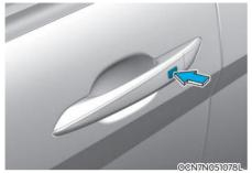
To lock the doors, press the button on the outside door handle while carrying the smart key with you or press the door lock button on the smart key.
