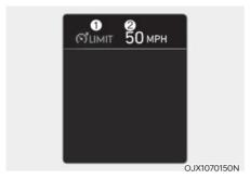
[1]: Manual Speed Limit Assist enabled indicator[2]: Set speedYou can set the speed limit when you do
