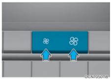
The fan speed can be set to the desired speed by using the fan speed control switch.
