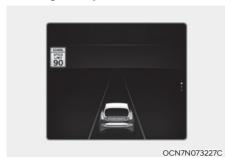
When driving at a speed higher than the displayed speed limit, the speed limit appears in red.
