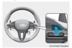
Press the Driving Assist () button to turn Cruise Control off. The Cruise () CRUISE) indicator will go off. Always press the Driving Assist () button to turn Cruise Control off when not in use.
