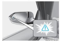
To warn the driver a vehicle is detected, the warning light on the side view mirror will illuminate.
