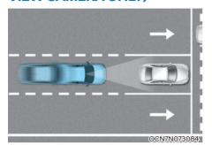
Forward Collision-Avoidance Assist helps detect a vehicle, a powered two-wheeler, a pedestrian, or a cyclist ahead on the road and may warn you of a possible collision with a warning message on the instrument cluster and a warning sound. Also, Forward Collision-Avoidance Assist may assist with braking your vehicle to help reduce collision speed or avoid a collision.
