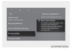
With the engine on, select Setup > Vehicle > Driver Assistance > Driving Safety > Blind-Spot Safety from the settings menu in the infotainment system. to set whether to use each function.
