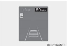
Manual Speed Limit Assist assists the vehicle to adjust its speed according to the speed limit. When the cruising speed is set as same as the speed limit, the vehicle automatically adjusts its speed if the speed limit changes. The function operates on the road which has a speed limit of 44 mph (70 km/h) or higher. When the function is active, the set speed on the instrument cluster appears in green.
