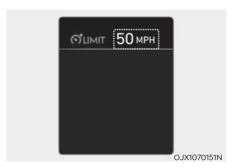
3. The set speed limit will be displayed on the instrument cluster.
