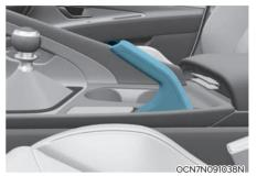
Check the stroke of the parking brake by counting the number of "clicks" heard while fully applying it from the released position. Also, the parking brake alone should securely hold the vehicle on a fairly steep grade. If the stroke is more or less than specified, have the system serviced by an authorized HYUNDAI dealer.
