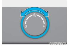
Turn the knob to the right to increase the fan speed and airflow. Turn the knob to the left to decrease fan speed and airflow.
