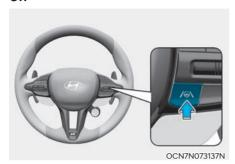
With the engine on, short press the Lane Driving Assist button located on the steering wheel to turn on Lane Following Assist. The white or green  $\bigcirc$  indicator light will illuminate on the instrument cluster.
