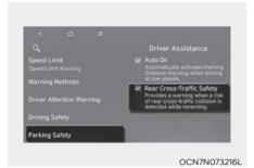
With the engine on, select Setup > Vehicle > Parking Safety > Rear Cross-Traffic Safety from the settings menu in the infotainment system to turn on Rear Cross-Traffic Collision-Avoidance Assist and deselect to turn off the function.
