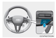
Press the II S switch to temporarily pause the set speed limit. The set speed limit will turn off but the Manual Speed Limit Assist (© LIMIT) indicator will stay on.
