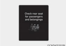
When the driver turns off the engine and opens the driver's door after opening and closing a rear door, a warning message "Check rear seat for passengers and belongings" appears on the cluster.
