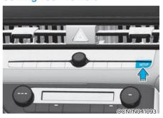
1. Press the SETUP button on the main keyboard.
