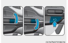
Operate the +, - switch or II button. If you push the + switch up or - switch down, vehicle speed will be set to the current speed on the instrument cluster.
