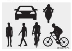
The illustration above shows the image the front view camera will detect as a vehicle, a powered two-wheeler, a pedestrian or a cyclist.
