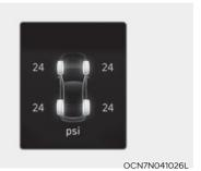
This warning message is displayed if the tire pressure is low. The corresponding tire on the vehicle will be illuminated.
