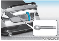
Open the trunk, and remove the towing hook from the tool case.
