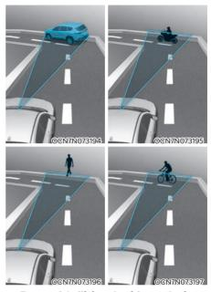
Forward Collision-Avoidance Assist may detect a vehicle, a powered two-wheeler, a pedestrian or a cyclist in the next lane or outside the lane when driving on a curved road. If this occurs, Forward Collision-Avoidance Assist may unnecessarily warn the driver and control the brake. Always check the traffic conditions around the vehicle.
