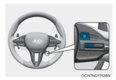
To change the trip mode, toggle the "\wedge, \widensighty" switch on the steering wheel.
