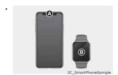
The NFC Antenna position on Apple iPhone is located at the top of the rear [A] and Apple WATCH is located at the center of the screen [B].
