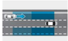
Blind-Spot Collision-Avoidance Assist helps detect and inform the driver that a vehicle is approaching at high speed from the blind spot area.
