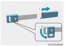
Turn the knob (2) of the mechanical key after removing the key protector (1). After using the mechanical key, turn the key knob (2) and insert the key protector (1).
