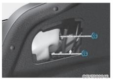
3. Loosen the assembly retaining nuts.
