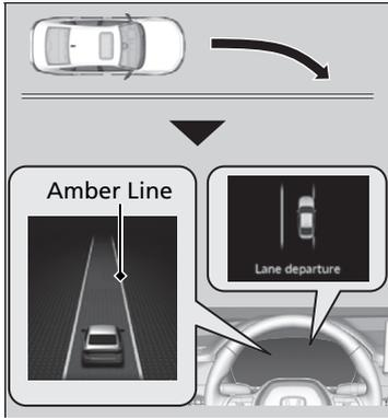
The front sensor camera behind the rearview mirror monitors left and right lane markings in white or yellow, the outer edge of the pavement (bordered by grass or gravel) or a detected oncoming vehicles.
