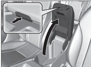
Push in the lock knob to open the console compartment.
