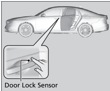
The vehicle will automatically lock after you lock the doors in advance then close the doors.
