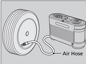
4. Recheck the air pressure using the air hose on the compressor.
