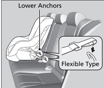
4. Attach the child seat to the lower anchors according to the instructions that came with the child seat.
