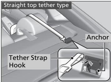
1. Locate the appropriate tether anchor point and lift the cover.
