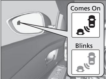
Blind spot information system alert indicator: Located on the outside door mirror on both sides.
