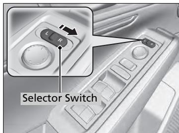
If activated, the passenger side door mirror automatically tilts downward when you put the transmission into **R**: this improves close-in visibility on the passenger side of the vehicle when backing up. The mirror automatically returns to its original position when you take the transmission out of **R**.
