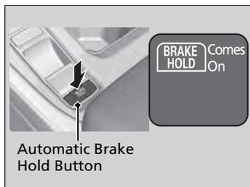
Fasten your seat belt properly, then start the power system. Press the automatic brake hold button.
