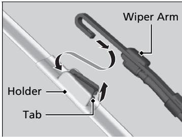
4. Press up on and hold the tab, then slide the holder off the wiper arm.
