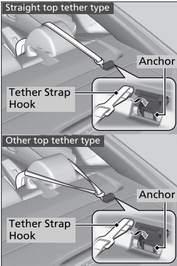
5. Open the tether anchor cover behind the head restraint.
