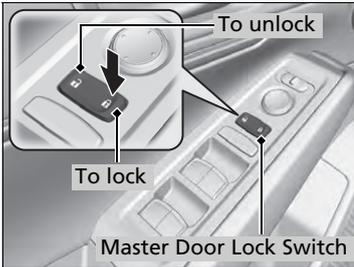
Press the master door lock switch in as shown to lock or unlock all the doors and fuel fill door.
