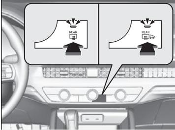
Press the rear defogger and heated door mirror\* button to defog the rear window and mirrors when the power mode is in ON.
