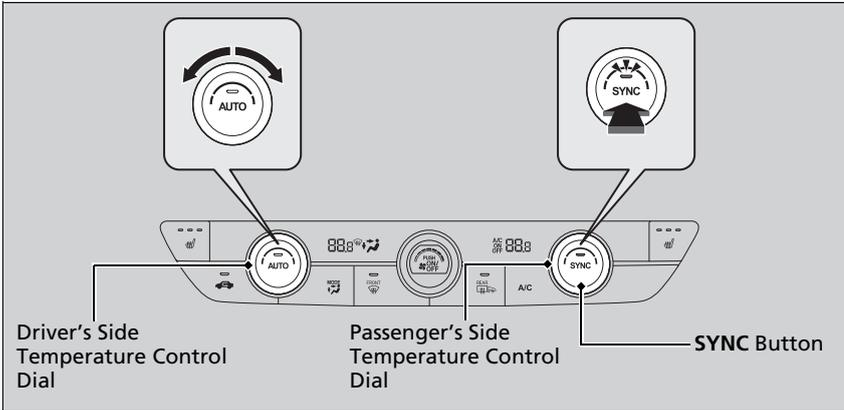
You can set the temperature synchronously for the driver's side and the passenger's side in synchronization mode.
