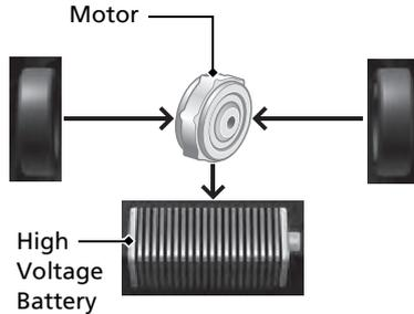
When decelerating without the accelerator being depressed or the brake pedal being applied, or while driving downhill, the electric motor acts as a generator that recovers a portion of the electrical energy that was used to accelerate the vehicle. This regenerative braking slows the vehicle in a manner similar to engine braking in a gasoline-powered vehicle.
