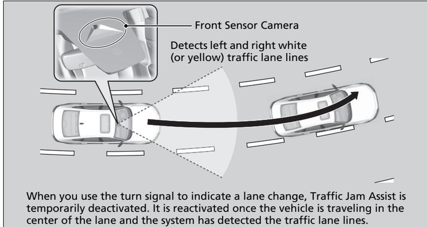
When the driver takes full control of the steering, the steering assist function is temporarily canceled.
