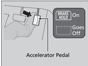
Depress the accelerator pedal while the shift lever is in a position other than **P** or **N**. The system is canceled and the vehicle starts to move.
