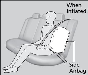
When the sensors detect a moderate-to-severe side impact, the control unit signals the side airbag on the impact side to immediately inflate.
