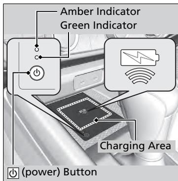
1. To turn the system on and off, press and hold the
