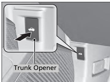
Pressing and holding the trunk opener under the driver's side lower corner of the dashboard unlocks and opens the trunk.
