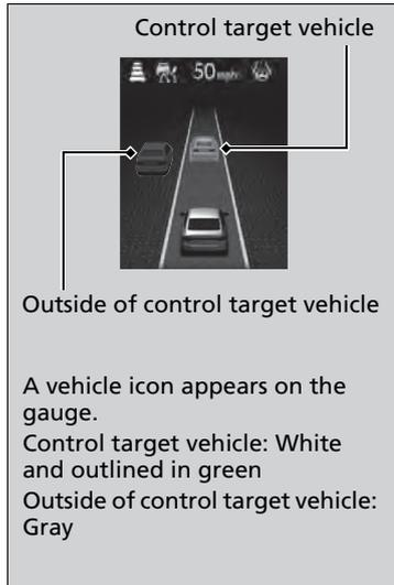
When a vehicle whose speed is slower than your set speed comes in or cuts in front of you and is detected by the radar and the camera, your vehicle starts to slow down.
