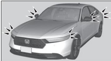
If the power system is turned off successfully, the exterior lights flash once.
