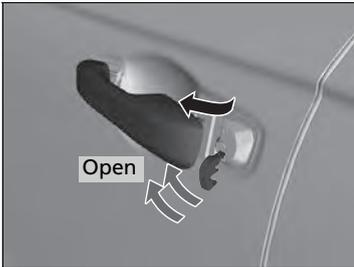
Pull and hold the outer handle. Completely insert the key into the key cylinder from below the handle.
