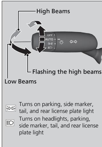
Rotating the light switch turns the lights on and off, regardless of the power mode setting.
