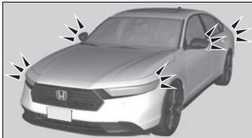
If the power system is turned on successfully, some exterior lights flash six times.
