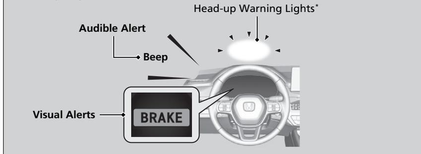
You can change the distance (**Long/Normal/Short**) between vehicles at which the system's earliest collision alert will come on through the audio/information screen setting options.
