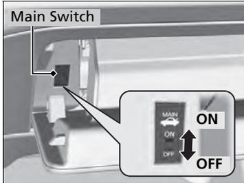
The trunk main switch disables the trunk release button on the remote transmitter, trunk release button on the trunk lid, and trunk opener under the driver's side lower corner of the dashboard to protect luggage in the trunk.
