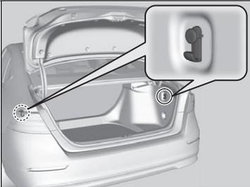
The cargo hook in the trunk can be used to install a net for securing items.
