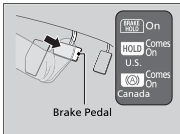
Depress the brake pedal to come to a complete stop. The shift lever must not be in **P** or **R**.
