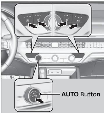
Press the seat heater or the seat ventilation button:
