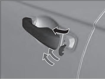
If the unlock button of the remote does not work, use the key instead. The keyhole is on the back of the door handle.
