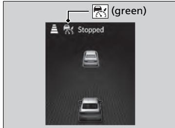
Your vehicle also stops, automatically. The **Stopped** message appears on the gauge. When the vehicle ahead of you starts again, if you press the **RES/+SET/-** switch up or down, or depress the accelerator pedal, ACC with Low Speed Follow will operate again within the prior set speed.
