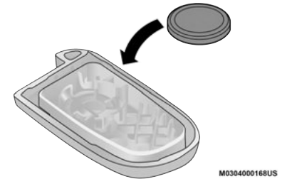
Key Fob Battery Replacement
