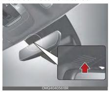
The auto defogging system oper-AUTO ates when the heater or air conditioning is on.
