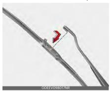
4. Make sure that both blade assemblies are installed firmly by trying to pull it slightly.
