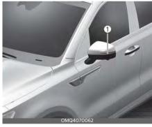
If the Side repeater lamp (LED) (1) does not operate, have your vehicle checked by a professional workshop.
