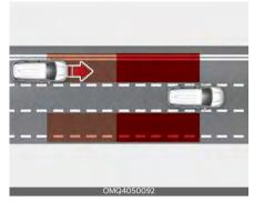
Blind-Spot Collision Assist help detect and informs the driver that a vehicle is approaching at high speed from the blind spot area.
