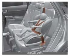
A forward-facing child seat provides restraint for the child's body with a harness. Keep children in a forward-facing child seat with a harness until they reach the top height or weight limit allowed by your child restraint's manufacturer.
