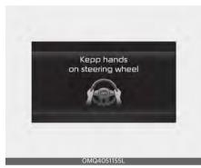
If the driver takes their hands off the steering wheel for several seconds, the 'Keep hands on the steering wheel' warning message will appear and an audible warning will sound in stages. First stage: Warning message Second stage: Warning message (red steering wheel) and audible warning
