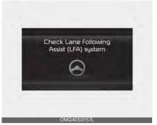
When Lane Following Assist is not working properly, the 'Check Lane Following Assist (LFA) system' warning message will appear on the cluster. If this occurs, have the function inspected by an authorized Kia dealer.
