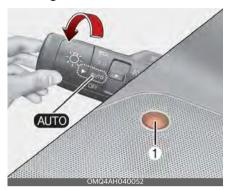
When the light switch is in the AUTO light position, the taillamps and head-lamps will turn ON or OFF automatically depending on the amount of light outside the vehicle.
