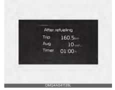
This display shows the trip distance, the average fuel efficiency, and the instant fuel efficiency (or the total driving time) since refueling.
