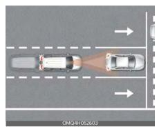
Forward Collision-Avoidance Assist is designed to help detect and monitor the vehicle ahead or help detect a pedestrian or cyclist in the roadway and warn the driver that a collision is imminent with a warning message and an audible warning, and if necessary, apply emergency braking.
