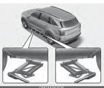
8. Insert the jack handle into the jack and turn it clockwise, raising the vehicle until the tire just clears the ground. This measurement is approximately 1.2 inches (30 mm). Before removing the wheel lug nuts, make sure the vehicle is stable and that there is no chance for movement or slippage.
