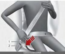
To fasten your seat belt, pull it out of the retractor and insert the metal tab (1) into the buckle (2). There will be an audible "click" when the tab locks into the buckle.
