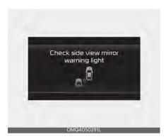
When the side view mirror warning light is not working properly, the 'Check side view mirror warning light' warning message will appear on the cluster. Have the function inspected by an authorized Kia dealer.
