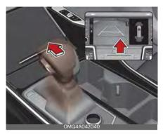
Rear View Monitor will show the area behind the vehicle to assist you when parking or backing up.
