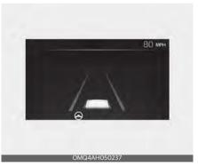
If the vehicle ahead and/or both lane markings are detected and your vehicle speed is above 60 km/h (40 mph) and below 200 km/h (120 mph), the green ( ) indicator light will appear on the
