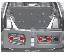
You can adjust the direction of air delivered from these vents using the vent control lever as shown.
