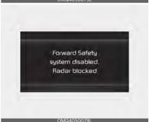
When the front windshield where the front view camera is located, front radar cover, sensor is covered with foreign material, such as snow or rain, it can reduce the detecting performance and temporarily limit or disable Forward Collision-Avoidance Assist.
