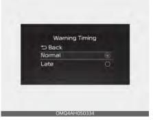
With the ENGINE START/STOP button in the ON position, select 'Driver Assistance → Warning Timing' from the Settings menu to change the initial warning activation time for Driver Attention Warning. When the vehicle is first delivered, Warning Timing is set to 'Normal'. If you change the Warning Timing, the warning time of other Driver Assistance systems may change.
