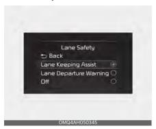
With the ENGINE START/STOP button in the ON position, select or deselect 'Driver Assistance → Lane Safety' from the Settings menu to set whether or not to use each function.
