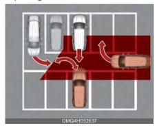
Rear Cross-Traffic Collision-Avoidance Assist may detect vehicles which are parking or pulling out near your vehicle (for example: a vehicle leaving
