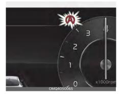
The engine will stop and the green AUTO STOP ((A)) indicator on the instrument cluster will illuminate.
