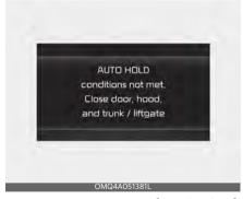
At this moment, press the [AUTO HOLD] button after closing the driver's door and engine hood.
