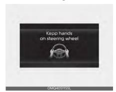
If the driver takes their hands off the steering wheel for several seconds, the 'Keep hands on the steering wheel' warning message will appear on the cluster, and an audible warning will sound in stages.
