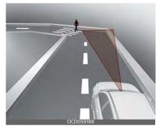
Forward Collision-Avoidance Assist may not detect other vehicles, pedestrians in front of you on curved roads adversely affecting the performance of the sensors. This may result in no warning, braking assist or steering assist when necessary.
