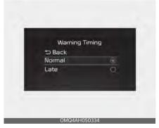
With the ENGINE START/STOP button in the ON position, select 'Driver Assistance → Warning Timing' from the Settings menu to change the initial warning activation time for Rear Cross-Traffic Collision-Avoidance Assist.
