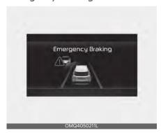
To warn the driver that emergency braking will be assisted, the 'Emergency Braking' warning message will appear on the cluster, an audible warning will sound, and the steering wheel will vibrate.
