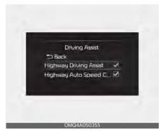
With the ENGINE START/STOP button in the ON position, select or deselect 'Driver Assistance → Driving Assist' from the Settings menu to set whether or not to use each function.
