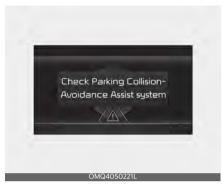
When Reverse Parking Collision- Avoidance Assist or other related systems are not working properly, the 'Check Parking Collision-Avoidance Assist system' warning message will appear on the cluster, and the function will turn off automatically. Have your vehicle inspected by an authorized Kia dealer.
