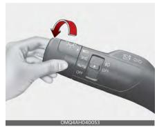
When the light switch is in the headlamp position, headlamp (low beam), tail, license light will turn ON.
