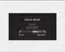
With the standard driving style in the center, the left side of the gauge is 'Econ.' and right side is 'Dynamic' style. When the left side of the driver's style gauge is filled up and after a certain time passes, the SMART ECO mode is activated automatically. When the right side of the gauge is filled up and sporty driving condition is detected, the SMART SPORT mode is activated.
