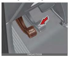
Check whether the stroke is within specification when the parking brake pedal is depressed with 30 kg (66 lbs., 294 N) of force. Also, the parking brake alone should securely hold the vehicle on a fairly steep grade. If the stroke is more or less than specified, have the system serviced by an authorized Kia dealer.
