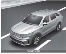
The front view camera is used as a detecting sensor to detect ambient light and brightness while driving.
