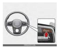
Press the Driving Assist ( MODE) button to turn Manual Speed Limit Assist off. The Speed Limit indicator ( UNIT) will go off.
