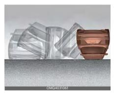
Airbags may not inflate if the vehicle collides with an object such as a utility pole or tree. This is because the point of impact is concentrated in one area and the full force of the impact is not delivered to the sensors.
