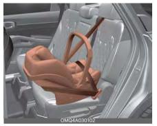
A rear-facing child seat provides restraint with the seating surface against the back of the child. The harness system holds the child in place, and in an accident, acts to keep the child positioned in the seat and reduces the stress to the neck and spinal cord.
