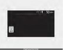
If the speed limit of the road changes during the operation of Manual Speed Limit Assist or Smart Cruise Control, an arrow in the direction of up or down is displayed to inform the driver that the set speed needs to be changed. At this time, the driver can change the set speed according to the speed limit by using the + or - switch on the steering wheel.
