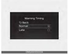
With the ENGINE START/STOP button in the ON position, select 'Driver Assistance → Warning Timing' from the Settings menu to change the initial warning activation time for Blind-Spot Collision-Avoidance Assist.
