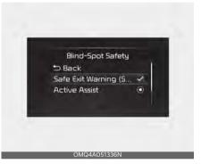
With the ENGINE START/STOP button in the ON position, select 'Driver Assistance → Blind-Spot Safety → Safe Exit Warning from the Settings menu to turn on Safe Exit Warning and deselect to turn off the function.
