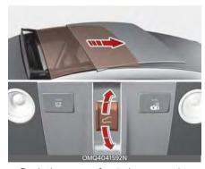
Push the sunroof switch rearward to the first detent position, the sunroof glass opens. However, if the power sunshade is close, the power sunshade will open first. Push the sunroof switch forward to the first detent position, the sunroof glass closes. However, if the sunroof glass is close, the power sunshade will close.
