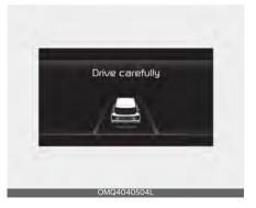
Navigation-based Smart Cruise Control is not able to slow down your vehicle to a safe speed
