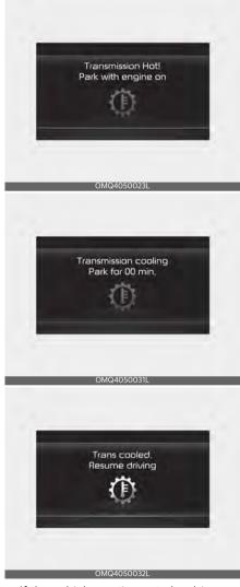
If the vehicle continues to be driven and the clutch temperatures reach the maximum temperature limit, the "Transmission Hot! Park with engine on" warning will be displayed. When this occurs the clutch is disabled until the clutch cools to normal temperatures.
