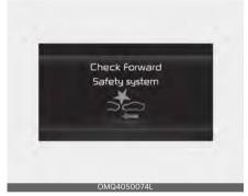
When Forward Collision-Avoidance Assist is not working properly, the 'Check Forward Safety system' warning message will appear, and the (/)) and
