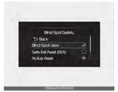
With the ENGINE START/STOP button in the ON position, select 'Driver Assistance → Blind-Spot Safety → Blind Spot View' from the Settings menu to turn on Blind-Spot View Monitor and deselect to turn off the function.
