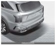
The wide-rear ultrasonic sensors are located inside the rear bumper to detect objects in the rear area. If the sensors are covered with foreign material, such as snow or rain, it may adversely affect sensor performance and Reverse Parking Collision-Avoidance Assist may not operate normally. Always keep the rear bumper clean.
