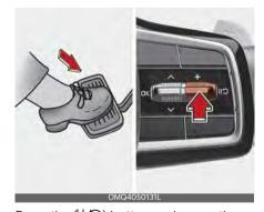
Press the (| ) button or depress the brake pedal to temporarily cancel Smart Cruise Control.
