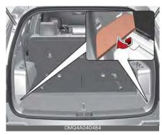
To open the cover, pull up the handle and lift the cover.
