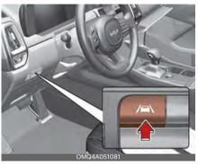
With the ENGINE START/STOP button in the ON position, press the Lane Safety button located on the instrument panel to turn on Lane Keeping Assist. The white ( ) indicator light will appear on the cluster.
