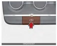
To change the air intake control position. Push the control button.
