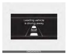
When the front vehicle departs from a stop, Leading Vehicle Departure Alert will inform the driver by displaying the 'Leading vehicle is driving away' message on the cluster and an audible warning will sound.
