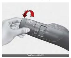
When the light switch is in the lamp position, the front position lamp, taillamp, and the license plate lamp will turn ON.
