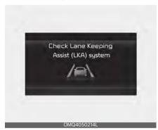
When Lane Keeping Assist is not working properly, the 'Check Lane Keeping Assist (LKA) system' warning message will appear and the yellow ( ) indicator light will appear on the cluster. If this occurs, have the function inspected by an authorized Kia dealer.
