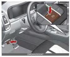
Releasing the parking brake with EPB switch.
