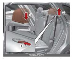
To remove the headrest, raise it as far as it can go then press the release button (1) while pulling the headrest up (2). To reinstall the headrest, put the headrest poles (3) into the holes while pressing the release button (1). Then adjust it to the appropriate height.
