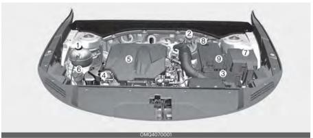
\* The actual engine room in the vehicle may differ from the illustration. 1. Engine coolant reservoir 7-18 7-21 2. Brake fluid reservoir 3. Air cleaner 7-23 7-16 4. Engine oil dipstick 5. Engine oil filler cap 7-16 6. Windshield washer fluid reservoir 7-22 7. Fuse box 7-48 8. Negative battery terminal 6-5, 7-29 9. Positive battery terminal 6-5, 7-29
