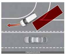
Blind-Spot Collision-Avoidance Assist may not operate properly when driving where the road merges or divides. The function may not detect the vehicle in the next lane.
