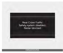
When the rear bumper around the rear corner radar or sensor is covered with foreign material, such as snow or rain, or installing a trailer or carrier, it can reduce the detecting performance and temporarily limit or disable Blind-Spot Collision-Avoidance Assist.
