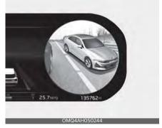
Blind-Spot View Monitor displays the rear blind spot area of the vehicle in the cluster when the turn signal is turned on to help safely change lanes.
