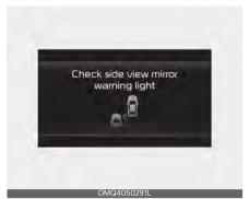
When the side view mirror warning light is not working properly, the `Check side view mirror warning light' warning message will appear on the cluster for several seconds, and the master ( \\_ \text{\Lambda}\)) warning light will appear on the cluster. If the master warning light appears, have the vehicle inspected by an authorized Kia dealer.
