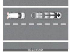
If the vehicle in front abruptly departures, Leading Vehicle Departure Alert may not operate properly.
