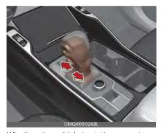
Whether the vehicle is stationary or in motion, manual mode is selected by pushing the shift lever from the D (Drive) position into the manual gate. To return
