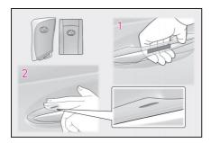
1 Grip the driver's door handle to unlock the door. Holding the driver's door handle for approximately 2 seconds unlocks all the doors. Grip any passenger door handle to unlock all the doors.\*
