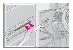
4 While pressing the "SET" button, or within 3 seconds after the "SET" button is pressed, press button "1", "2" or "3" until the buzzer sounds.
