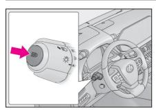
1 Press the Automatic High Beam switch.
