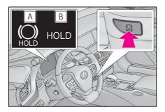
Turns the brake hold system on
