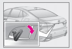
Turn the mechanical key clockwise to open.
