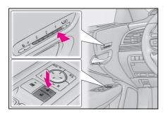
4 While pressing the recalled button, press and hold the door lock switch (either lock or unlock) until the buzzer sounds.
