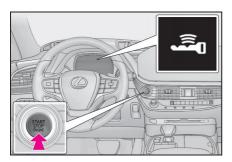
**3** Press the engine switch shortly and firmly.
