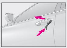
Pull the driver's door handle and insert the mechanical key
