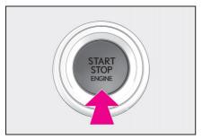
4 To stop the engine, press and hold the engine switch for 2 consecutive seconds or more, or press it briefly 3 times or more in succession.
