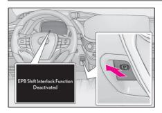
While the vehicle is stopped, pull and hold the parking brake switch until a message is shown on the multi-information display.
