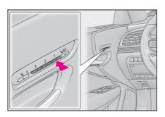
3 Press one of the buttons for the driving position you want to recall until the buzzer sounds.
