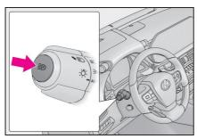
Press the Automatic High Beam switch.
