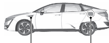
Hydrogen Ventilation Duct (Above the both front tires)
