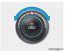
The fan speed can be set as desired by turning the fan speed control knob.
