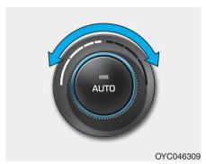
2. Turn the temperature control knob to the desired temperature. If the temperature is set to the lowest setting (Lo), the air conditioning system will operate continuously. After the interior has cooled sufficiently, adjust the knob to a higher temperature set point whenever possible.
