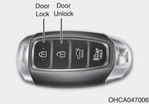
Press the button on the driver's outside door handle while carrying the Smart Key with you or press the Door Unlock button on the Smart Key, the driver's door will unlock. If you press the button on the front passenger's
