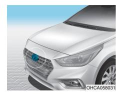
In order for FCA to operate properly, always make sure the sensor cover or sensor is clean and free of dirt, snow, and debris. Dirt, snow, or foreign substances on the sensor cover or sensor may adversely affect the sensing performance of the sensor.
