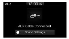
Connect the external device connection jack to the AUX terminal to run AUX.
