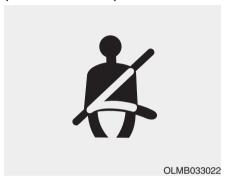
As a reminder to the driver, the seat belt warning light will illuminate for approximately 6 seconds each time you place the ignition switch to the ON position regardless of belt fastening. However, if the seat belt is unfasted, a warning chime will sound for approximately 6 seconds.
