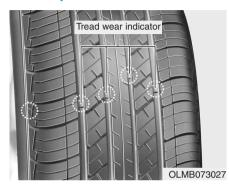
If the tire is worn evenly, a tread wear indicator will appear as a solid band across the tread. This shows there is less than 2/32 inch (1.6 mm) of tread left on the tire. Replace the tire when this happens.
