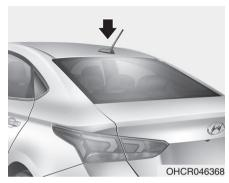
The roof antenna receives AM/FM signals.
