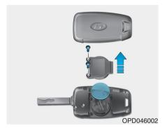
Battery Type: CR2032 To replace the battery:
