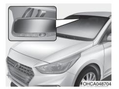
Auto defogging reduces the possibility of fogging up the inside of the windshield by automatically sensing the moisture on inside the windshield.
