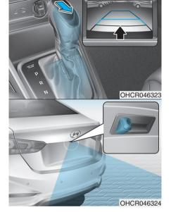
Rear View Monitor will activate when the engine is running and the shift lever is in the R (Reverse) position. This is a supplemental system that helps provide a view of the area behind the vehicle through the audio display while the vehicle is in the R (Reverse) position.
