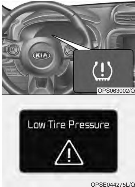
(1) Low tire pressure telltale / TPMS malfunction indicator
