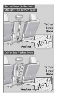
**3.** Secure the tether strap hook to the anchor.
