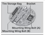
The tire storage bag, bracket, mounting wing bolt (A) and mounting wing bolt (B) are in the tool case.
