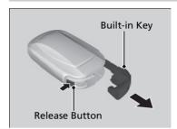
The built-in key can be used to lock/unlock the doors when the keyless remote battery becomes weak and the power door lock/unlock operation is disabled.
