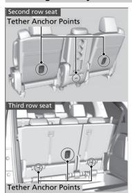
A tether anchor point is provided behind each second and third row seating position. If you have a child seat that comes with a tether but can be installed with a seat belt, the tether may be used for additional security.
