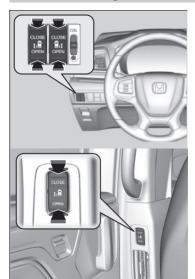
The power sliding door opens when you press the **OPEN** side of the [18] / [21] switch, and closes when you press the **CLOSE** side of the [18] / [21] switch.
