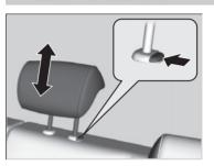
A passenger sitting in the second row/third row center seating position should adjust the height of their head restraint to an appropriate position before the vehicle begins moving.
