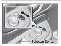
If activated, either side door mirror automatically tilts downward when you put the transmission into  $\boxed{\mathbf{R}}$ ; this improves close-in visibility on the selected side of the vehicle when backing up. The mirror automatically returns to its original position when you take the transmission out of  $\boxed{\mathbf{R}}$ .
