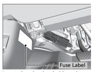
Located under the dashboard. Fuse locations are shown on the label on the side panel.
