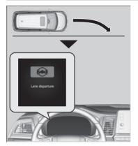
The front camera behind the rearview mirror monitors left and right lane markings (in white or yellow). If your vehicle is getting too close to detected lane markings without a turn signal activated, the system, in addition to a visual alert, applies steering torque and alerts you with rapid vibrations on the steering wheel, to help you remain within the detected lane.
