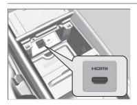
There is an HDMI<sup>TM</sup> port in the console compartment. The rear entertainment system will accept HDMI<sup>TM</sup> cable connections with video equipment that is equipped with an HDMI<sup>TM</sup> port.
