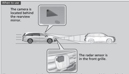
The system starts monitoring the roadway ahead when your vehicle speed is about 3 mph (5 km/h) or above and there is a vehicle in front of you.
