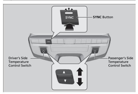
You can set the temperature synchronously for the driver's side, the passenger's side and the rear passenger compartment in synchronization mode.
