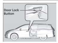
The vehicle will automatically lock after you lock the doors in advance then close the passenger's door, power sliding doors, and tailgate.
