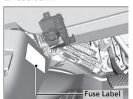
Located under the dashboard. Fuse locations are shown on the label on the side panel.
