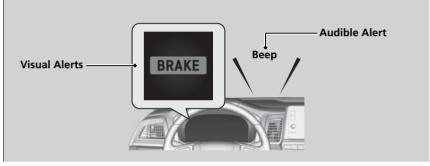
You can change the distance (**Long/Normal/Short**) between vehicles at which the system's earliest collision alert will come on.
