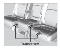
A transceiver is installed in second row removable seats to wirelessly communicate the seat belt fastening information to the vehicle. It will automatically connect to the vehicle whenever the seats is in or near its installation position.
