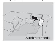
Gently depress the accelerator pedal. When on a hill, it may require more accelerator input to release.
