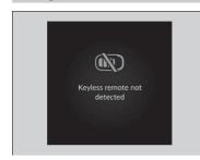
When the power mode is set to any mode other than OFF and you remove the keyless remote from the vehicle and shut the door, an alarm will sound. If the alarm continues to sound, place the keyless remote in another location.
