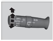
The lights will turn on automatically depending on the ambient brightness. They can also be switched on and off manually.
