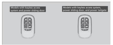
Use the keys to start and stop the engine, and lock and unlock all the doors, tailgate, and fuel fill door
