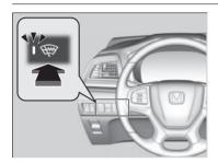
Press the heated windshield button to deice the windshield at the wiper park area and along the driver side edge of the windshield when the power mode is in ON. The heated windshield will automatically switch off after 15 minutes.
