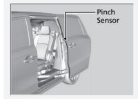
Do not touch the pinch sensor located at the front edge of the power sliding door. Do not damage the sensor. The power sliding door may not operate properly.
