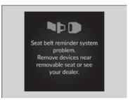
If the vehicle loses connection with any transceiver while the seat belt is fastened, the information for that seat will change to unfastened, and a "Seat belt reminder system problem" warning will be displayed. When any seat is not installed, please ensure that the seat belt does not remain fastened in order to prevent lost communication with the transceiver.
