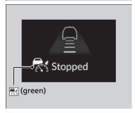
If no vehicle is ahead of you before you resume driving, depressing the accelerator pedal will resume operation of ACC with Low Speed Follow within the prior set speed.
