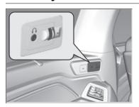
The headphone connector for the rear entertainment system is on the left side of the third row outer seats. The connector has its own volume control.
