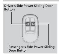
Press the power sliding door button for more than one second to operate.
