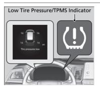
Monitors the tire pressure while you are driving. If your vehicle's tire pressure becomes significantly low, the Low Tire Pressure/TPMS indicator comes on and a message appears on the driver information interface.
