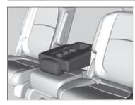
Pull up the strap and fold down the center backrest to use as an armrest.
