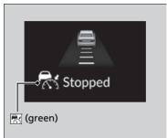
Your vehicle also stops, automatically. The **Stopped** message appears on the gauge. When the vehicle ahead of you starts again, if you press the **RES/+/SET/-** switch up or down, or depress the accelerator pedal, ACC with Low Speed Follow operates again within the prior set speed.
