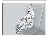
If a lap/shoulder seat belt cannot be used properly, position the child in a booster seat in the rear seat. For the child's safety, check that the child meets the booster seat manufacturer's recommendations.
