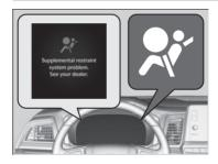
■ When the power mode is set to ON The indicator comes on for a few seconds, then goes off. This tells you the system is working properly.
