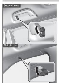
There are coat hooks under the grab handles in the second row, and under the window frames in the third row. Pull it down to use it.
