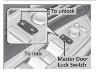
Press the master door lock switch in as shown to lock or unlock all doors, tailgate, and fuel fill door.
