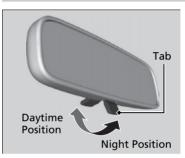
Flip the tab to switch the position. The night position will help reduce the glare from headlights behind you when driving after dark.
