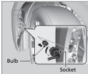
Turn the steering wheel all the way to the opposite side from the light being replaced.
