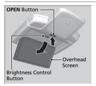
Push the **OPEN** button, then pull down the screen to the first or second detent until it latches.
