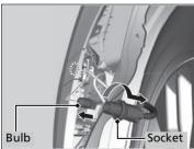
Turn the steering wheel all the way to the opposite side from the light being replaced.
