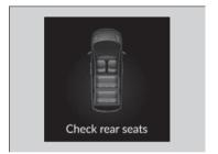
A reminder appears on the driver information interface and an alert will sound when the power mode is set to VEHICLE OFF.
