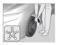
**5.** Lower the vehicle and remove the jack. Tighten the wheel nuts in the order indicated in the image. Go around tightening the nuts two to three times in this order.
