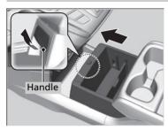
To open the console box, pull the handle and slide the box forward.
