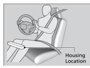
The knee airbag for the driver and the one for the front passenger are housed under the steering column and the glove box respectively.
