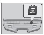
Press the rear defogger and heated door mirror button to defog the rear window and mirrors when the power mode is in ON.
