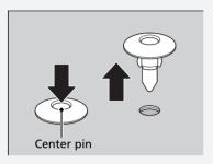
Push the center pin back to lock the clip. Then, insert the clip into the hole and press on the center pin until it is flat.
