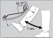
Use a forward and back kicking motion for about 1 second under the center of the rear bumper to open or close the power tailgate while carrying the keyless remote.
