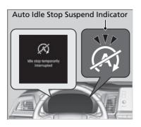
The Auto Idle Stop suspend indicator comes on and a message appears on the driver information interface when the Auto Idle Stop system cannot be activated.
