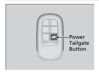
Press the power tailgate button for more than one second to operate when the power mode is in VEHICLE OFF.
