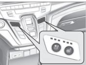
Press the seat heater or the seat ventilation button:
