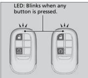
Press the <u>a</u> button, then press and hold the <u>D</u> button.
