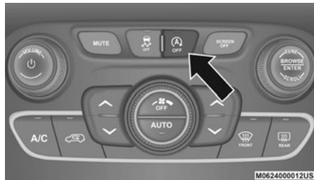
Stop/Start OFF Switch
