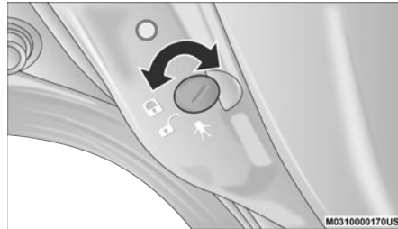
Child-Protection Door Lock Location
