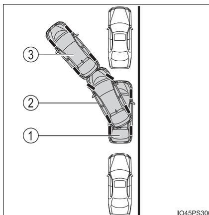
Depending on the condition of the parking space, guidance to starting points for moving forward and backing up, as well as the steering wheel auto operation, are repeated any time multi-turn maneuvering is necessary from the time the steering wheel auto operation begins in step ② up until the vehicle reaches a position from which it can take off.
