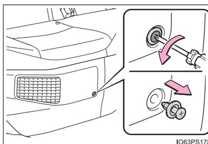
**3** Remove the air intake vent cover.
