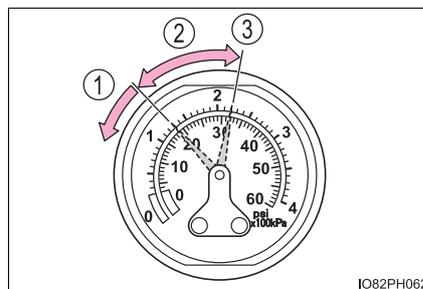
22 Turn the compressor switch on to inflate the tire until the specified air pressure is reached. Drive for about 3 miles (5 km) and then perform step 20.
