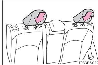
■ Adjusting the height of the head restraints (front seats)
