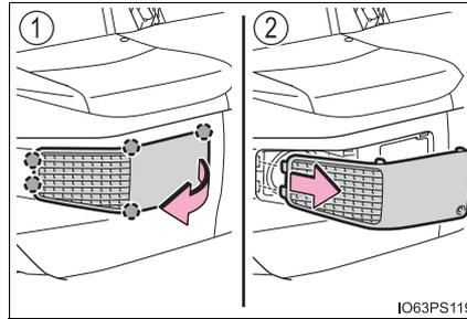
**4** Remove the air intake vent filter.
