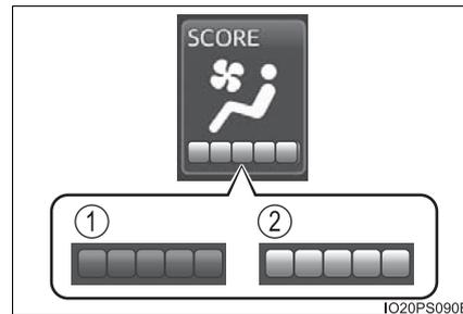
\*1: The Eco score (A/C score) is not evaluated for approximately 1 minute after the power switch is turned to ON mode.
