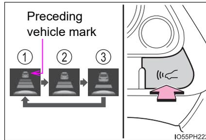
**Vehicle-to-vehicle distance settings (vehicle-to-vehicle distance control mode)**
