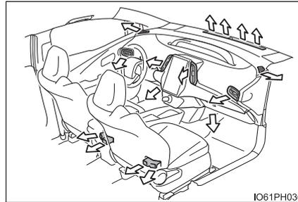
■ **Adjusting the air flow direction**
