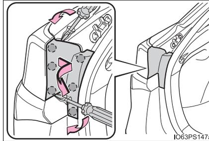
To prevent damage to the cover, protect the tip of the screwdriver with a rag.
