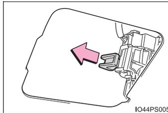
Using the lever to open the fuel filler door may not allow for an adequate reduction in fuel tank pressure before refueling. To prevent fuel from spilling out, turn the cap slowly when removing it.
