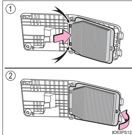
**7** Install the air intake vent cover.
