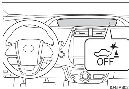
When the Parking Support Brake function is switched off, system operation does not resume until the function is switched back on through the
