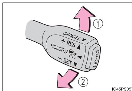
Large adjustment: Hold the lever up or down to change the speed, and release when the desired speed is reached.
