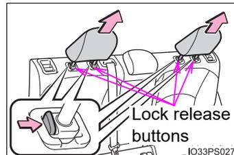
■ **Installing the head restraints**
