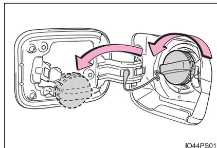
■ **When the fuel filler door cannot be opened by pressing the inside switch**
