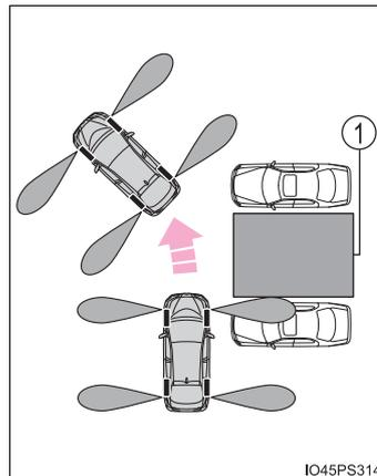
● The sensor detection range when using parallel parking assist mode
