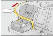
S While pushing the child restraint system into the rear seat, allow the shoulder belt to retract until the child restraint system is securely in place.
