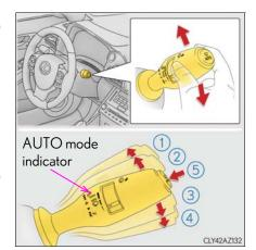
With AUTO mode selected, the wipers will operate automatically when the sensor detects falling rain. The system automatically adjusts wiper timing in accordance with rain volume and vehicle speed.
