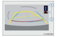
A simplified image is displayed on the upper part of the screen when an obstacle is detected.
