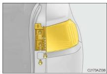
Push and pull the light unit toward the rear of the vehicle as shown in the illustration to remove it.
