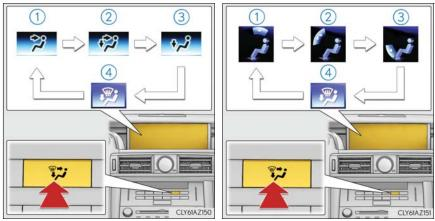
The air outlets used are switched each time the button is pressed.
