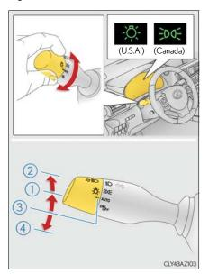
1 With the headlights on, push the lever away from you to turn on the high beams.
