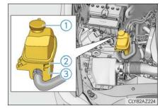
Only use "Toyota Super Long Life Coolant" or a similar high quality ethylene glycol based non-silicate, non-amine, non-nitrite, and non-borate coolant with long-life hybrid organic acid technology.
