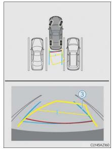
Once the vehicle width guide lines and the parking space lines are parallel, straighten the steering wheel and back up slowly until the vehicle has completely entered the parking space.
