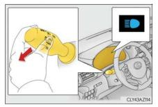
**2** Press the Automatic High Beam switch.
