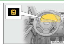
If the vehicle gets stuck in mud, dirt or snow, the TRAC system may reduce power from the engine to the wheels. Pressing to turn the system off may make it easier for you to rock the vehicle in order to free it.
