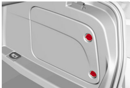
Battery Access Panel
