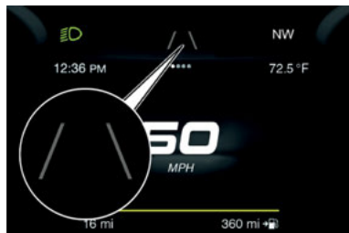
Lane Markings Not Detected
