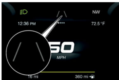
Lane Markings Not Detected
