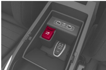
Center Console Power Outlet
