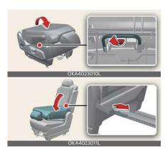
Pull the removal strap or lever and lift the rear portion of the seat cushion. Then the rear catches will be released. Remove the seat while lifting the rear portion of seat cushion and then reinstalling the tumble seat.
