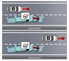
[A]: Approaching car from side Lane-Change Side function can help mitigate or avoid a collision with vehicles or powered two-wheelers in the next lane when changing lanes by assisting the driver's steering.
