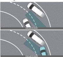
Blind-Spot Collision-Avoidance Assist may not operate properly on a curved road. Blind-Spot Collision-Avoidance Assist may not detect the vehicle in the next lane.
