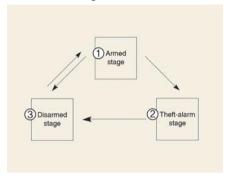
If triggered, the system provides an audible alarm with blinking of the haz ard warning lights.
