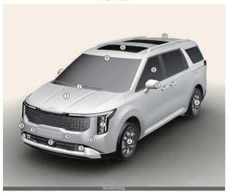
\* The actual shape of your Kia may differ from the illustration. 1. Hood 5-62 2. Head lamp 5-119, 9-50 3. Front fog lamp 9-50 4. Wheel and tire 9-27, 10-5 5. Outside rearview mirror 5-89 6. Sunroof 5-67 5-124, 9-24 7. Front windshield wiper blades 8. Windows 5-57 7-112 9. Front ultrasonic sensor 10.Front radar 7-4 11. Front view camera 7-4
