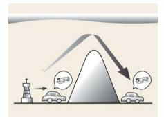
AM broadcasts can be received at greater distances than FM broadcasts. This is because AM radio waves are transmitted at low frequencies. This long distance, low frequency radio waves can follow the curvature of the earth rather than traveling straight. In addition, they curve around obstructions resulting in better signal coverage.
