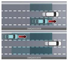
Blind-Spot Collision-Avoidance Assist can help detect and inform the driver that a vehicle is approaching at high speed from the blind spot area.
