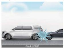
Front airbags may not inflate in side impact collisions, because passen gers move in the direction of the collision. In side impacts, frontal airbag deployment would not provide additional occupant protection.
