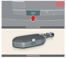
1 Power liftgate open/close button see Press the power liftgate open/close but ton for 1 second. The liftgate opens or closes with a warning sound.
