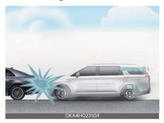
Front air bags may inflate in a frontal collision depending on several factors, including the severity, speed and angles of impact.
