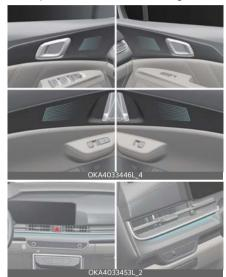
When the headlamp light is on, the ambient light is on at the same time could be set in the infotainment menu. Refer to the infotainment manual for details.
