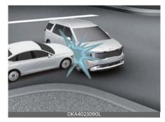
In an angled collision, the force of impact may direct the occupants in a direction where the air bags would not be able to provide any additional benefit, and the sensors may not deploy any air bags.
