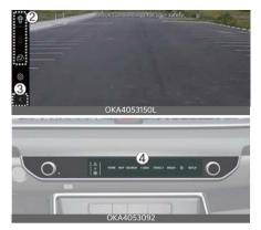
The front-view function displays the vehicle's front situation on the navigation system according to the driver's settings, assisting in safe driving.
