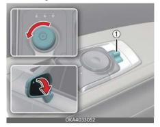
The position of the outside rear view mirror select switch (1) determines whether the mirrors will move:
