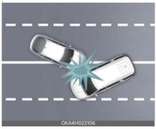
Just before an impact, drivers may brake heavily. Such heavy braking may lower the front portion of the vehicle causing it to "ride" under a vehicle with a higher ground clear ance. Air bags may not inflate in this "under-ride" situation because deceleration forces that are detected by sensors may be significantly reduced by such "under-ride" collisions.
