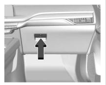
Lift the handle to open the glove box. Close until it latches. Use the vehicle key to lock or unlock. See  $Keys \Rightarrow 6$ .
