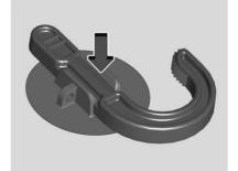
2. Push down on the other side of the load floor hook to lock into place.
