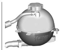
3. If topping off the level in the coolant surge tank, add the proper mixture until the level reaches the mark on the front of the tank and replace the cap. Operate the vehicle. Repeat steps 1–3, as necessary.
