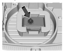
Turn the retainer nut counterclockwise to remove the tire sealant and compressor kit bag. 5. Remove the tire sealant and compressor kit from the bag.
