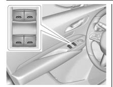
The power windows work when the ignition is on, in ACC/ACCESSORY, or when Retained Accessory Power (RAP) is active. See *Retained Accessory Power (RAP)* ⇒ 223.
