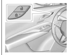
**a**: Press to lock the doors. The indicator light in the switch will illuminate when locked.
