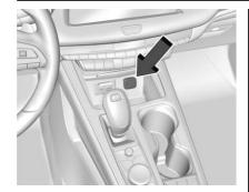
The vehicle has three accessory power outlets: one at the front of the center console, one under the armrest, and one in the rear cargo area.
