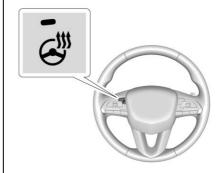
②: If equipped, press to turn on or off. A light near the button displays when the feature is turned on.
