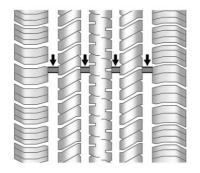
Treadwear indicators are one way to tell when it is time for new tires. Treadwear indicators appear when the tires have only 1.6 mm (1/16 in) or less of tread remaining. See *Tire Inspection*  $\Rightarrow$  322 and *Tire Rotation*  $\Rightarrow$  323 for additional information.
