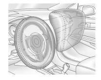
The driver frontal airbag is in the center of the steering wheel.
