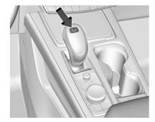
**P**: This position locks the drive wheels. Use P (Park) when starting the engine to prevent the vehicle from moving easily.
