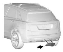
To remove hitch cover, if equipped:
