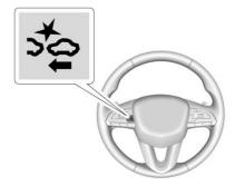
The Collision Alert control is on the steering wheel. Press to set the FCA timing to Far, Medium, or Near. The first button press shows the
