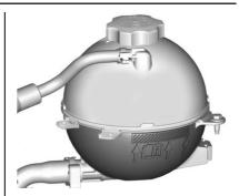
Check to see if coolant is visible in the coolant surge tank. If the coolant inside the coolant surge tank is boiling, do not do anything else until it cools down. If coolant is visible but the coolant level mark is not at or above the indicated mark, add a 50/50 mixture of clean, drinkable water and DEX-COOL coolant. Be sure the cooling system is cool before this is done. See *Engine Overheating* ⇔ 294.
