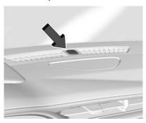
There is a light sensor on top of the instrument panel. Do not cover the sensor.
