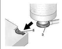
5. Slide the base of the tire sealant canister (3) into the slot on the top of the compressor (6) to hold it upright.
