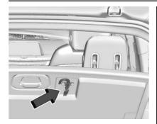
To install the load floor hook into the holder:
