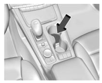
4. Place the new transmitter into the front cupholder.
