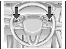
If equipped, vehicles with Tap Shift have controls on the back of the steering wheel to manually shift the automatic transmission.
