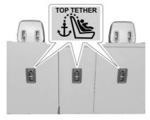
The top tether anchors are on the back of the rear seatbacks. Remove the cargo cover before installing the top tether. The cargo cover can be replaced after the top tether is properly installed. Be sure to use an
