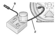
Attach the sealant/air hose (2) to the tire valve stem by turning it clockwise until tight. 8. Plug the power plug (9) into the accessory power outlet in the vehicle. Unplug all items from other accessory power outlets. See *Power Outlets* ⇔ 95.
