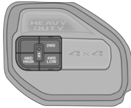
Four-Position/Part-Time Transfer Case
