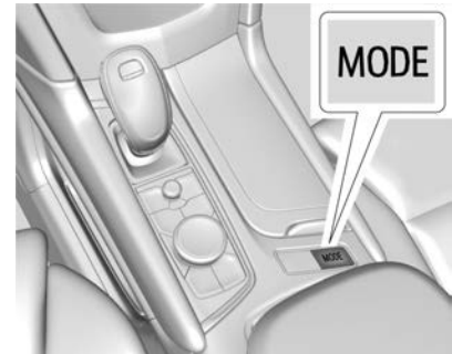
Driver Mode Control Switch
