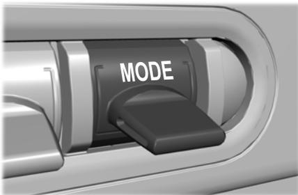
To change the drive mode setting, press the mode button on the instrument panel under the display. The first press illuminates the selected mode, subsequent presses change the selected mode.
