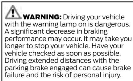
**WARNING:** Driving your vehicle with the warning lamp on is dangerous. A significant decrease in braking performance may occur. It may take you longer to stop your vehicle. Have your vehicle checked as soon as possible. Driving extended distances with the parking brake engaged can cause brake failure and the risk of personal injury.
