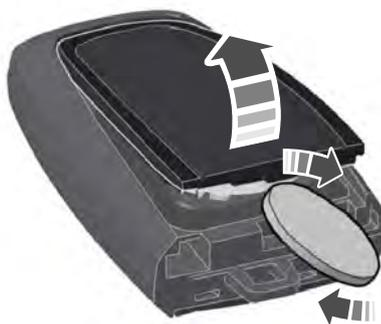
2. Twist a thin coin under the tab hidden behind the key blade head to remove the battery cover.
