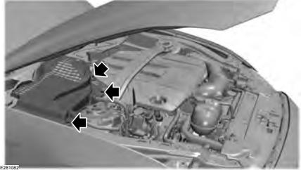
1. Rotate and release three fasteners by hand from the battery shield.
