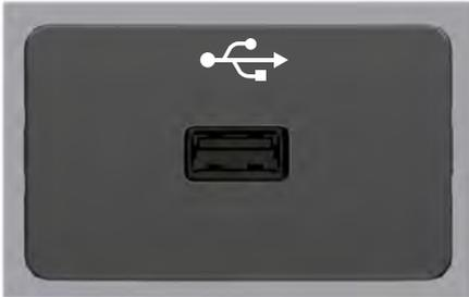
The USB port allows you to plug in media playing devices, memory sticks and charge devices.
