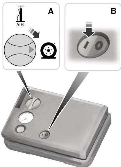
7. Turn dial (A) clockwise to the sealant position. Switch the kit on by pressing the on/off button (B).
