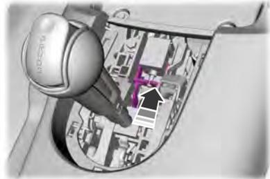
2. Locate the white release lever and slide the lever forward when pulling the gearshift lever out of the park (P) position and into the neutral (N) position.
