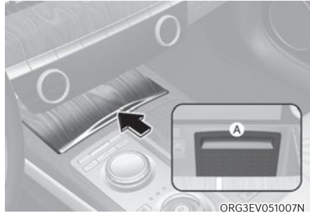
[A] : In-vehicle authentication pad (Wireless charging pad)
