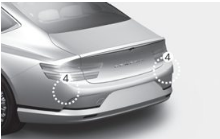
[1]: Front view camera, [2]: Front radar, [3]: Front corner radar (if equipped), [4]: Rear corner radar
