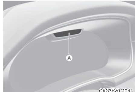
[A] : Interior view camera
