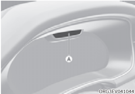
[A] : Interior view camera
