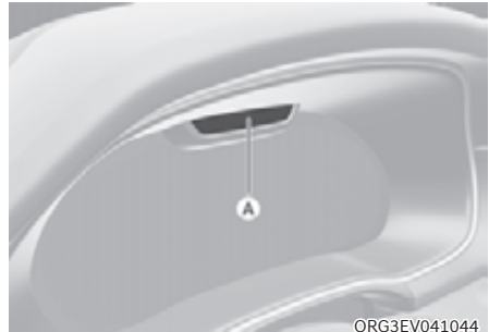
[A] : Interior view camera
