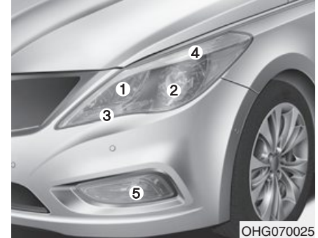
Headlight, position light, turn signal light, front fog light bulb replacement
