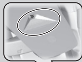
■ Front Sensor Camera Monitors the lane lines
