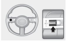
Press the (IIO) switch to temporarily pause the set speed limit. The set speed limit will turn off but the Speed Limit (STLIMIT) indicator will stay on.
