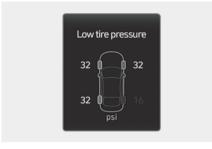
This warning message appears if the tire pressure is low. The corresponding tire on the vehicle is illuminated.
