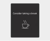
The "**Consider taking a break**" message will appear and the inattentive driving (造) warning light will blink on the instrument cluster with a warning sound to suggest that the driver take a break, when the driver's attention level is below a certain level.
