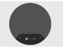
The fuel gauge indicates the approximate amount of fuel remaining in the fuel tank.
