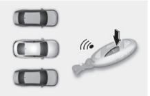
2. Press and hold the Remote Start button (ഹ) within 4 seconds until the engine starts.
