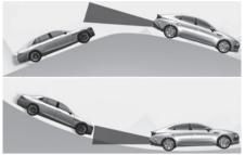
Blind-Spot Collision-Avoidance Assist may not operate properly when driving on a slope. The function may not detect the vehicle in the next lane or may incorrectly detect the ground or structure. Always pay attention to road and driving conditions while driving.
