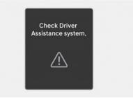
When Lane Following Assist is not working properly, the **Check Driver Assistance system.** warning message will appear on the instrument cluster for several seconds, and the master (A) warning light appears on the instrument cluster. If this occurs, have your vehicle inspected by an authorized HYUNDAI dealer.
