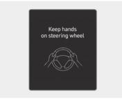
If the driver takes their hands off the steering wheel for several seconds, the "**Keep hands on steering wheel**" warning message appears on the instrument cluster, and an audible warning sounds in stages.
