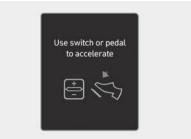
When Highway Driving Assist is operating, your vehicle will stop if the vehicle ahead of you stops. Also, if the vehicle ahead of you starts moving within 30 seconds after the stop, your vehicle will start as well. In addition, after the vehicle has stopped and 30 seconds have passed, the "**Use switch or pedal to accelerate**" message will appear on the instrument cluster. Depress the accelerator pedal or operate the + switch, - switch or (**IIO**) switch to start driving.
