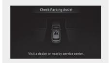
When Remote Smart Parking Assist is not working properly, the "**Check Parking Assist**" warning message will appear on the infotainment system. If the message appears, stop using Remote Smart Parking Assist, and we recommend that your vehicle be inspected by an authorized HYUNDAI dealer. **Remote Smart Parking Assist cancelled**
