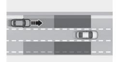
Blind-Spot Collision-Avoidance Assist helps detect and informs the driver that a vehicle is approaching at high speed from the blind spot area.
