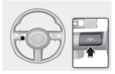
With the engine on, shortly press the Lane Driving Assist button located on the steering wheel to turn on Lane Following Assist. The gray or green  $(\Theta)$  indicator light will appear on the instrument cluster.
