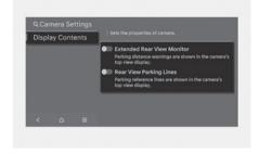
You can change Rear View Monitor **Display Contents** by touching the setup icon (尊) on the screen while rear view Monitor is operating, or selecting **Setup** > **Vehicle > Driver Assistance > Parking Safety > Camera Settings** from the Settings menu in the infotainment system while the engine is on.
