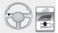
2. Push the + switch up or - switch down, and release it at the desired speed.
