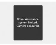
When the front windshield where the front view camera is located is covered with foreign material, such as snow or rain, it can reduce the detecting performance and temporarily limit or disable Intelligent Speed Limit Assist. If this occurs, the "**Driver Assistance system limited. Camera obscured.**" warning message and the speed limit ( $\square$ ) warning light will appear on the instrument cluster.
