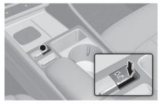
Press and hold the Parking Safety (Pm) button more than 2 seconds, to turn the Parking Collision-Avoidance Assist on or off.
