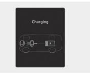
The engine and regenerative brake system charges up the high voltage battery. (Engine and Wheel  $\rightarrow$  Battery)
