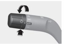
Hight Beam Assist automatically switches between high beam and low beam depending on the detected brightness from the lights of oncoming vehicles or vehicles in front.
