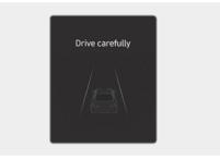
When the vehicle is stopped due to emergency braking, the "Drive carefully" warning message will appear on the instrument cluster.
