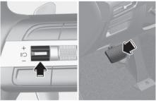
Press the (IIO) switch or depress the brake pedal to temporarily cancel Smart Cruise Control.
