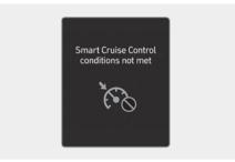
If the Driving Assist button, + switch, switch or (IIO) switch is operated when Smart Cruise Control operating conditions are not satisfied, the "Smart Cruise Control conditions not met" will appear on the instrument cluster, and an audible warning will sound.
