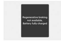
Regenerative braking is temporarily limited to protect the battery because the high voltage battery is fully charged.
