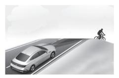
Forward Collision-Avoidance Assist may not detect a vehicle, a powered two-wheeler, a pedestrian, or a cyclist in front of you while driving uphill or downhill, adversely affecting the performance of the sensors.
