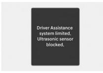
If this occurs the "**Driver assistance** system limited. Ultrasonic sensor blocked" warning message appears on the instrument cluster. Parking Distance Warning operates properly when snow, rain or foreign material is removed. If Parking Distance Warning does not operate properly after obstruction (snow, rain, or foreign material) is removed (including trailer, carrier, etc., from the rear bumper), have your vehicle inspected by an authorized HYUNDAI dealer.
