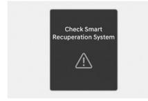
If the rear radar is covered by any foreign material, such as snow, rain, or dirt, the detecting performance may decrease and disable the smart recuperation system.
