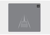
If the vehicle ahead and/or both lane markings are detected and your vehicle speed is below 120 mph (200 km/h), the green  $(\Theta)$  indicator light appears on the instrument cluster, and Lane Following Assist helps center the vehicle in the lane by assisting the steering wheel.
