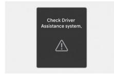
When Blind-Spot Collision-Avoidance Assist is not working properly, the "**Check Driver Assistance system.**" warning message will appear on the instrument cluster for several seconds, and the master ((A)) warning light will appear on the instrument cluster. If this occurs, have your vehicle inspected by an authorized HYUNDAI dealer.
