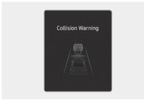
To warn the driver of a collision, the **"Collision Warning**" warning message appears and the ( $\stackrel{<}{\Rightarrow}$ ) warning light blinks on the instrument cluster with a warning sound and the steering wheel vibrates.
