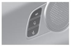
The IMS, or Integrated Memory System, for the driver's seat is provided to store and recall the following memory settings with a simple button operation.
