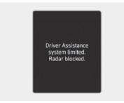
When the front radar cover or sensor is covered with snow, rain, or foreign material, it can reduce the detecting performance and temporarily limit or disable Smart Cruise Control.
