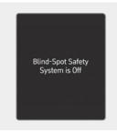
When the vehicle is restarted with Blind-Spot Collision-Avoidance Assist off, the "**Blind-Spot Safety System is Off**" message will appear on the instrument cluster.
