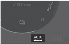
The smart recuperation system is ON and the regenerative braking level appears as **"AUTO**".
