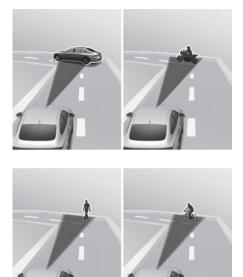
Forward Collision-Avoidance Assist may detect a vehicle, powered two-wheeler, pedestrian, or cyclist in the next lane or outside the lane when driving on a curved road.
