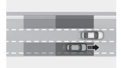
Blind-Spot Collision-Avoidance Assist helps detect and informs the driver that a vehicle is in the blind spot.
