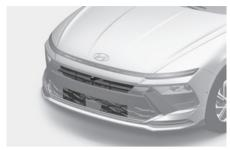
Active air flap system controls the air flap below the front bumper to cool the vehicle parts and improve fuel economy.
