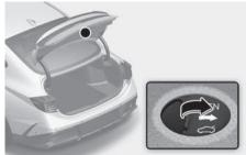
Your vehicle is equipped with the emergency trunk safety release lever located on the bottom of the trunk.
