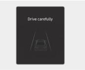
When the vehicle is stopped due to emergency braking, the "Drive carefully" warning message will appear on the instrument cluster.
