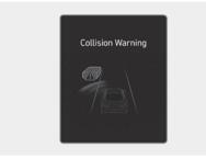
To warn the driver of a collision, the "**Collision Warning**" warning message appears and the ( $\stackrel{<}{\rightarrow}$ ) warning light blinks on the instrument cluster with a warning sound and the steering wheel vibrates.
