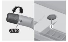
The parking light and headlight are turned ON or OFF automatically depending on the amount of daylight as measured by the ambient light sensor (1) in front of the instrument panel.
