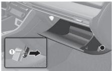
2. Press both sides of the glove box inward to release.
