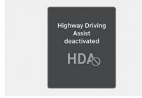
If the driver still does not have their hands on the steering wheel after the hands-off warning, "**Highway Driving Assist deactivated**" warning message will appear and Highway Driving Assist will be automatically canceled.
