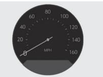
The speedometer indicates the speed of the vehicle and is calibrated in kilometers per hour (km/h) and/or miles per hour (MPH).
