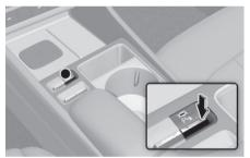
Press the Parking Safety (P∞) button to turn on Parking Distance Warning. Press the button again to turn off the function.
