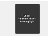
When the side view mirror warning light is not working properly, the "**Check side view mirror warning light**" warning message will appear on the instrument cluster for several seconds, and the master warning light ( $\triangle$ ) will appear on the instrument cluster. If this occurs, have your vehicle inspected by an authorized HYUNDAI dealer.
