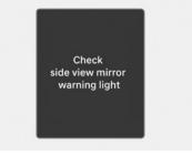
When the side view mirror warning light is not working properly, the "**Check side view mirror warning light**" warning message appears on the instrument cluster for several seconds, and the master (A) warning light illuminates on the instrument cluster. If this occurs, have your vehicle inspected by an authorized HYUNDAI dealer.
