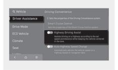
With the engine on, select or deselect Setup > Vehicle > Driver Assistance > Driving Convenience from the Settings menu to set whether to use each function. If "**Highway Driving Assist**" is selected, it helps maintain distance from the vehicle ahead, maintain the set speed, and helps center the vehicle in the lane.
