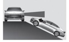
Rear Cross-Traffic Collision-Avoidance Assist may be limited when the vehicle is on a uphill or downhill slope, or near it, and may not detect the vehicle approaching from the left or right. If this occurs, the function may not warn the driver or control the brakes when necessary.
