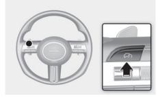
Press the Driving Assist ( ) button to turn Manual Speed Limit Assist off. The Speed Limit ( ) LIMIT) indicator will go off.
