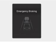
To warn the driver that emergency braking will be assisted, the "**Emergency Braking**" warning message appears and the (♣) warning light blinks on the instrument cluster with a warning sound and the steering wheel vibrates.
