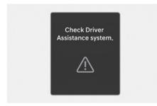
When Forward Collision-Avoidance Assist is not working properly, the "Check Driver Assistance system." warning message will appear, and the (A), (李) warning light will illuminate on the instrument cluster. Have your vehicle inspected by an authorized HYUNDAI dealer.
