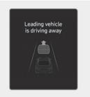
When a detected vehicle in front departs from a stop, Leading Vehicle Departure Alert will inform the driver by displaying the "Leading vehicle is driving away" message on the instrument cluster and an audible warning will sound.
