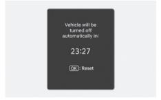
When all the conditions are satisfied, the Vehicle Auto-Shut Off operates and turns the engine off automatically after 60 minutes.
