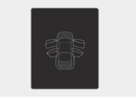
This warning appears if any door or hood or trunk is left open. The warning indicates which door is open on the cluster display.
