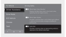
With the engine on, select **Setup** > **Vehicle** > **Driver Assistance** > **Driving Safety** > **Safe Exit** from the Settings menu to turn on Safe Exit Warning and deselect to turn off the function.
