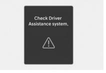
When Highway Driving Assist is not working properly, the "Check Driver Assistance system." warning message and yellow Lane Keeping Assist (/=\) warning light appears on the instrument cluster. If this occurs, have your vehicle inspected by an authorized HYUNDAI dealer.
