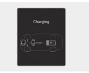
The engine is simultaneously used to drive the vehicle and to charge up the high voltage battery.
