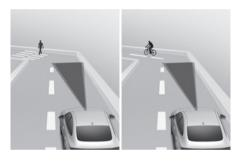
Forward Collision-Avoidance Assist may not detect a vehicle, a powered two-wheeler, a pedestrian, or a cyclist in front of you when driving on curved roads adversely affecting the performance of the sensors. This may result in no warning, braking assist when necessary.
