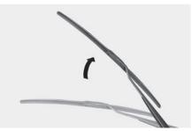
3. Lift up the wiper blade clip (1). Then pull down the wiper blade (2). Remove the wiper blade from the wiper arm.
