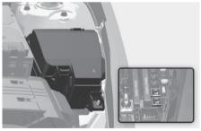
5. Pull the suspected fuse straight out. Use the removal tool (1) provided in the engine compartment fuses panel cover.
