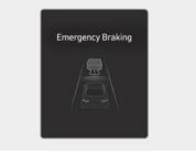
To warn the driver that emergency braking will be assisted, the "**Emergency Braking**" warning message appears and the (♣) warning light blinks on the instrument cluster with a warning sound and the steering wheel vibrates. In emergency braking situation, braking is assisted with strong braking power to help prevent collision with the oncoming vehicle.
