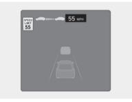
Manual Speed Limit Assist or Smart Cruise Control assists the vehicle to adjust its speed according to the speed limit. When the cruising speed is set as same as the speed limit, the vehicle automatically adjusts its speed if the speed limit changes. The function operates on the road which has a speed limit of 45 mph (70 km/h) or higher. When the function is active, the cruising speed on the instrument cluster appears in green.
