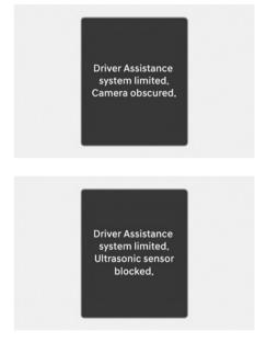
The "Driver Assistance system limited. Camera blocked." or "Driver Assistance system limited. Ultrasonic sensor blocked." warning message will appear on the cluster if the following situations occur:
