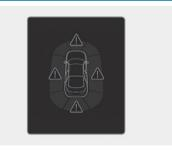
When the Parking Distance Warning is operating, if the function is not working normally or the ultrasonic sensor is blocked, the master warning light (A) appears in the direction of the corresponding sensor. You can check the warning in the Utility view on the cluster.
