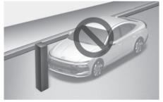
Remote Smart Parking Assist performance may reduce or collision with an obstacle may occur when there is a narrow object, circular pillar, square pillar, or a pillar surrounded by objects such as a fire extinguisher, etc., near the parking space. The driver should park the vehicle manually. • Parking in a parking space with a vehicle on one side only
