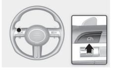
To turn Smart Cruise Control off, press the Driving Assist (ශා) button.
