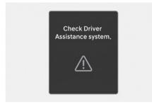
When Driver Attention Warning is not working properly, the "**Check Driver Assistance system.**" warning message will appear on the instrument cluster for several seconds, and the master (A) warning light and the inattentive driving (D) warning light will appear on the instrument cluster. If this occurs, have your vehicle inspected by an authorized HYUNDAI dealer.
