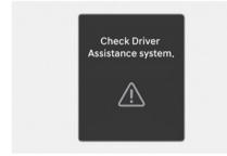
When Smart Cruise Control is not working properly, the "**Check Driver Assistance system.**" warning message and the master (<u>A</u>) warning light will appear on the instrument cluster. Have your vehicle inspected by an authorized HYUNDAI dealer.
