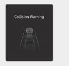
To warn the driver of a collision, the "**Collision Warning**" warning message appears and the (ﷺ) warning light blinks on the instrument cluster with a warning sound and the steering wheel vibrates.
