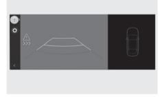
To warn the driver of an approaching vehicle from the rear left/right side of your vehicle, the warning light on the side view mirror blinks and a warning message appears on the instrument cluster. At the same time, an audible warning sounds and the steering wheel vibrates. A warning also appears on the infotainment system.
