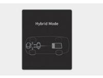
Both the motor and the engine power are used to drive the vehicle. (Battery & Engine  $\rightarrow$  Wheel)
