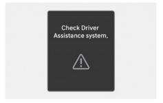
When Safe Exit Warning is not working properly, the "**Check Driver Assistance system.**" warning message will appear on the instrument cluster for several seconds, and the master warning light (<u>A</u>) will appear on the instrument cluster. If this occurs, have your vehicle inspected by an authorized HYUNDAI dealer.
