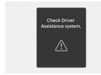
When Lane Keeping Assist is not working properly, the "**Check Driver Assistance system.**" warning message and yellow Lane Keeping Assist (/=\) warning light appears on the instrument cluster. If this occurs, have your vehicle inspected by an authorized HYUNDAI dealer.
