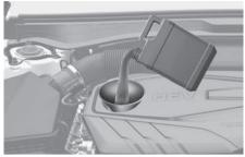
Use only the specified engine oil (Refer to the "Recommended lubricants and capacities" section in chapter 2).
