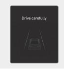
When the vehicle is stopped due to emergency braking, the "**Drive carefully**" warning message will appear on the instrument cluster.
