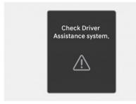
When Intelligent Speed Limit Assist is not working properly, the "Check Driver Assistance system." warning message will appear on the instrument cluster for several seconds, and the master (A) warning light and speed limit () warning light will appear on the instrument cluster. If this occurs, have your vehicle inspected by an authorized HYUNDAI dealer.
