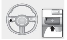
Press the button repeatedly to cycle through the headway settings from Distance 4 > Distance 3 > Distance 2 > Distance 1 > Distance 4.
