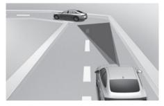
On curves, Smart Cruise Control may not detect a vehicle in the same lane, and may accelerate to the set speed. Also, vehicle speed may rapidly decrease when the vehicle ahead is detected suddenly.
