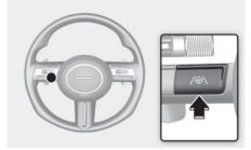
With the engine on, press and hold the Lane Driving Assist (/<sup>(-</sup>)) button located on the steering wheel to turn on and off. When Lane Keeping Assist is on, the (/=\) indicator is on.
