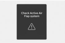
The active air flap system may not operate normally if the air flap is temporarily opened due to foreign factors or if the controller is contaminated by snow or rain, etc.
