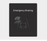
To warn the driver that emergency braking will be assisted, the "**Emergency Braking**" warning message appears and the (ﷺ) warning light blinks on the instrument cluster with a warning sound and the steering wheel vibrates. In emergency braking situation, braking is assisted with strong braking power to help prevent collision with the oncoming vehicle.
