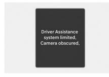
When the front windshield where the front view camera is located, or sensor is covered with foreign material, such as snow or rain, it can reduce the detecting performance and temporarily limit or disable Lane Keeping Assist.
