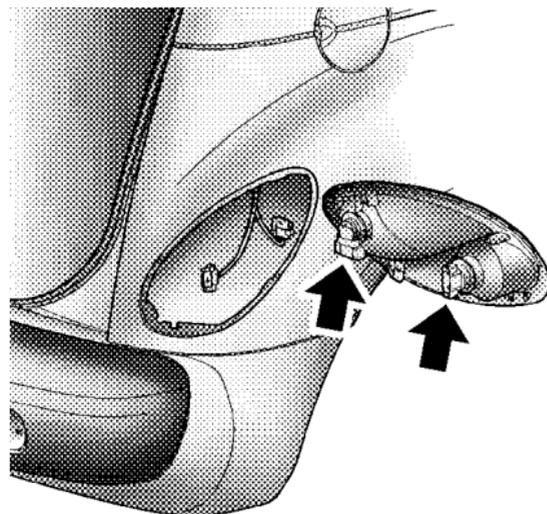
3. Pull the bulb out of the socket and replace.
