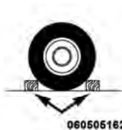
6. Block both the front and rear of the wheel diagonally opposite the jacking position. For example, if changing the right front tire, block the left rear wheel.
