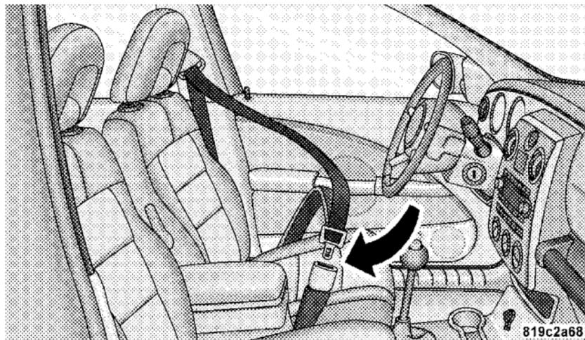
Inserting Latch Plate Into Buckle
