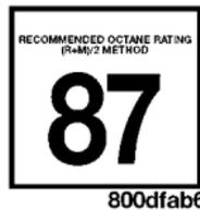
2.4L standard engines are designed to meet all emission regulations and provide excellent fuel economy and performance when using high quality unleaded “regular” gasolines having an octane rating of 87.
