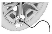
6. With the compressor switched off, insert the connector into the power socket in the vehicle interior.
