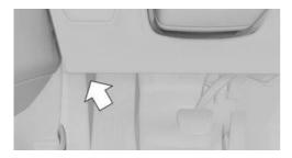
On the driver's side, there is a diagnostic socket for reading out vehicle data.
