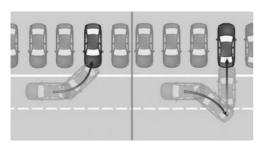
Perpendicular parking: reverse or forward parking perpendicular to the road.
