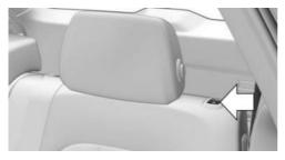
Pull the switch and fold the rear seat backrest forward.
