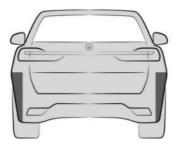
The radar sensors are located on the side of the rear bumper.
