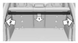
Pull out the cargo cover, arrow 1, and hook both sides onto the brackets, arrows 2.
