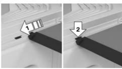
To restore the operability, close the cargo cover by hand, arrow 1, until it engages in the mounting, arrow 2.
