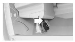
Slide the fragrance cartridge into the cartridge holder at a slight angle without applying pressure. The fragrance cartridge is correctly positioned when the cartridge holder can be closed.
