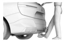
Before the cargo area opens, the hazard warning system flashes.
