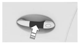
Hold the smartphone NFC antenna directly at the center of the driver's door handle. The position of the near field communication antenna depends on the smartphone model.
