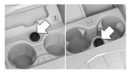
A socket is located between the cup holders in one of the marked positions. Detach the cover.
