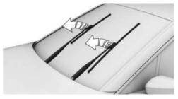
3. Press the button, arrow 1, turn the wiper blade slightly clockwise, and pull it forward and out, arrow 2.
