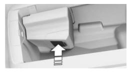
Remove the cover of the new fragrance cartridge. Hold the cover on the top to slide it from the fragrance cartridge.
