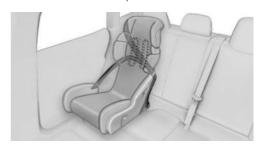
To secure child restraint systems, the rear seat belts and front passenger seat belt can be locked to prevent them from being pulled out.
