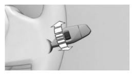
Turn the thumbwheel on the wiper lever.
