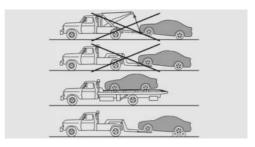
Have vehicle transported on a loading platform or use a tow dolly.
