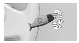
Turn the outer switch upward.
