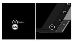
The note about a route section ahead is made as recommendation to let the vehicle coast to a halt.
