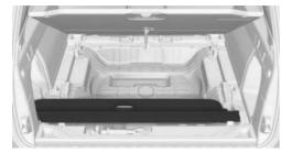
5. Push the cargo area floor down and close the storage compartment on the left side.
