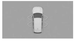
The maximum opening angle of the doors is displayed in selector lever position P.
