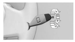
Turn the outer switch upward.
