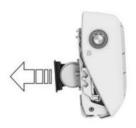
3. Remove the battery from the battery hous-
