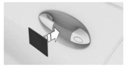
Hold the activated Key Card directly at the center of the driver's door handle.
