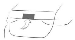
▶ Unlock the vehicle and then press the button on the cargo area.
