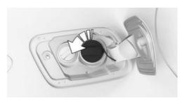
3. Place the fuel filler cap in the bracket on the fuel filler flap.
