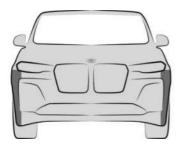
The radar sensors are located on the side of the front bumper.
