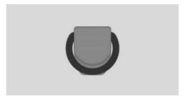
The lashing eyes are located in the cargo area. The front lashing eyes are located under covers.
