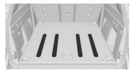
The system prevents slipping of the cargo in the cargo area when the anti-slip tracks are extended to the top.
