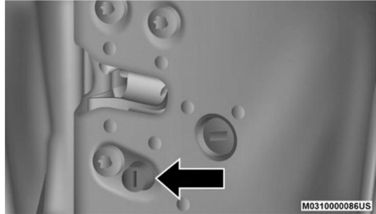
**Child Lock System****To Engage Or Disengage The Child-Protection Door Lock System**
