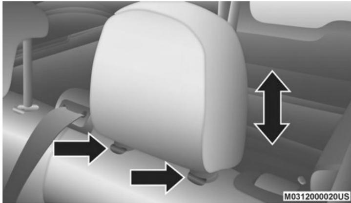
Outboard Head Restraint Release Buttons
