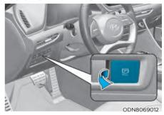
To apply the EPB (Electronic Parking Brake):
