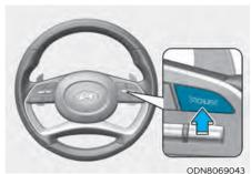
Pushing the CRUISE/ 5 button. The cruise indicator will go off. If you wish not to use the cruise control system, always turn the system off by pushing the CRUISE/ (5) button.
