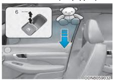
If a window senses any obstacle while it is closing automatically, it will stop and lower approximately 12 inches (30 cm) to allow the object to be cleared.
