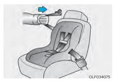
4. Slowly allow the shoulder portion of the seat belt to retract and listen for an audible "clicking" or "ratcheting" sound. This indicates that the retractor is in the "Automatic Locking" mode. If no distinct sound is heard, repeat steps 3 and 4.
