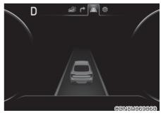
To see LKA screen on the LCD display in the cluster, select Driving Assist mode (A). For more information, refer to "LCD Display Modes" section in chapter 4.
