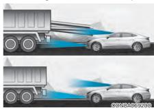
If the vehicle in front of you has cargo that extends rearward from the cab, or when the vehicle in front of you has higher ground clearance, additional special attention is required. FCA system may not be able to detect the cargo extending from the vehicle. In these instances, you must maintain a safe braking distance from the rearmost object, and if necessary, depress the brake pedal to reduce your driving speed in order to maintain distance.
