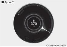
The hybrid system gauge indicates whether the current driving condition is fuel efficient or not.
