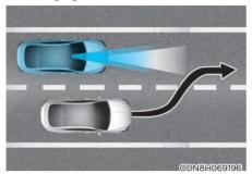
When a vehicle changes lanes in front of you, FCA system may not immediately detect the vehicle, especially if the vehicle changes lanes abruptly. In this case, you must maintain a safe braking distance, and if necessary, depress the brake pedal to reduce your driving speed in order to maintain a safe distance.
