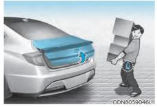
On a vehicle equipped with a smart key, the trunk can be opened using the Smart Trunk with Auto Open system.
