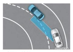
BCW and BCA systems may not operate properly when driving on a curved road. In certain instances, the system may recognize a vehicle in the same lane.
