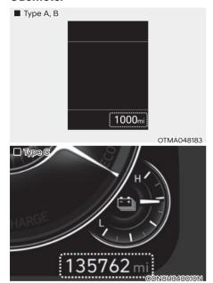
The odometer indicates the total distance that the vehicle has been driven and should be used to determine when periodic maintenance should be performed.
