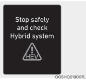
This message is displayed when there is a problem with the hybrid control system. The "\(\frac{1}{4}\)" indicator will blink and a warning chime will sound until the problem is solved. Refrain from driving when the warning message is displayed.
