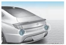
The rear corner radars are the sensors inside the rear bumper for detecting the side and rear areas. Always keep the rear bumper clean for proper operation of the system.
