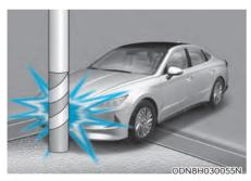
Air bags may not inflate if the vehicle collides with objects such as utility poles or trees, where the point of impact is concentrated and the collision energy is absorbed by the vehicle structure.
