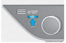
If you press the DRIVER ONLY button (\$\mathbb{G}^{DRIVER}\)) and the indicator light illuminates, air mostly blows in the direction of the driver's seat.
