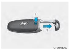
To remove the mechanical key from the smart key FOB, slide the release lever in the direction of the arrow (1) and then pull the mechanical key (2) outward.
