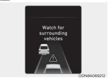
If the vehicle ahead (vehicle speed: less than 20 mph (30 km/h)) disappears to the next lane, the warning chime will sound and a message "Watch for surrounding vehicles" will appear. Adjust your vehicle speed for vehicles or objects that can suddenly appear in front of you by depressing the brake pedal.
