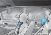
Your vehicle is equipped with a side air bag in each front seat and outboard rear seats. The purpose of the air bag is to provide the vehicle's driver and the front passenger with additional protection than that offered by the seat belt alone.
