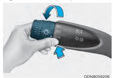
High Beam Assist is a system that automatically adjusts the headlamp range (switches between high beam and low beam) according to the brightness of other vehicles and road conditions.
