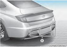
[A]: Front sensor, [B]: Rear sensor
