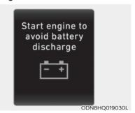
If the engine is not turned on with the Engine Start/Stop button in ACC or ON for a while, the battery can be discharged. Please turn on the engine to prevent 12V battery from discharge.
