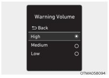
The driver can select the warning volume of Forward Collision Warning in the User Settings in the LCD display or infotainment system display by selecting 'User Settings → Driver Assistance → Warning Volume → High/Medium/Low'.
