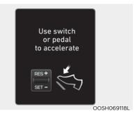
Use switch or pedal to accelerate
