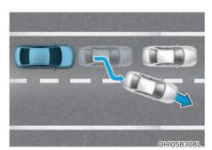
When driving in stop-and-go traffic, and a vehicle in front of you merges out of the lane, FCA system may not immediately detect the new vehicle that is now in front of you. In this case, you must maintain a safe braking distance, and if necessary, depress the brake pedal to reduce your driving speed in order to maintain a safe distance.
