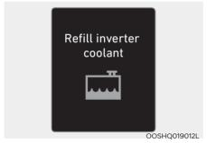
This message is displayed when the inverter coolant is nearly empty.
