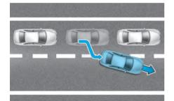
When driving in stop-and-go traffic, and a vehicle in front of you merges out of the lane, the system may not immediately detect the new vehicle that is now in front of you. In this case, you must maintain a safe braking distance, and if necessary, depress the brake pedal to reduce your driving speed in order to maintain a safe distance.
