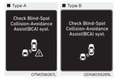
Check Blind-Spot Collision-Avoidance Assist (BCA) system
