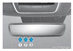
Press and release the programed HomeLink button to activate the garage door. 4. Once the garage door is stopped, press and release the "Learn" or "Smart" button on the Garage door opener within 1 minute from the time of pressing the programed HomeLink button on mirror.
