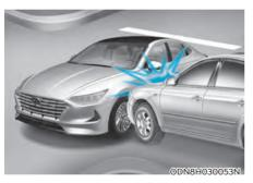
Front air bags may not inflate in side impact collisions, because occupants move in the direction of the collision, and thus in side impacts, front air bag deployment would not provide additional occupant protection.
