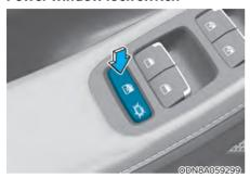
The driver can disable the power window switches on the rear passenger doors by pressing the power window lock switch. When the power window lock switch is pressed:
