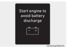
This message is displayed to inform the driver the 12V battery may be discharged if the ignition switch is in ON position (without the indicator ON).
