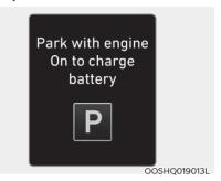
This message is displayed when the hybrid battery power (SOC) level is low.
