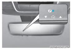
If the both indicator (4) and (6) are flashing rapidly for about 5 seconds, the two way synchronization is completed.
