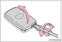
Remove the depleted battery.
