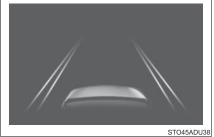
Indicates that the system is not able to recognize white (yellow) lines or is temporarily canceled. Lane departure alert function
