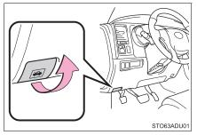
2 Pull up the hood catch lever and lift the hood.
