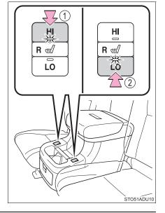
■ The seat heaters/seat ventilators can be used when The engine switch is in ON.
