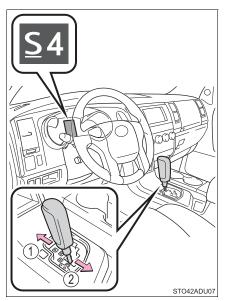
The initial shift range in S mode is set automatically to 5 or 4 according to vehicle speed. However, the initial shift range may be set to 3 if AI-SHIFT has operated while the shift lever was in the D position.  $(\rightarrow P. 222)$
