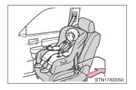
Vehicles with bench type second seats: When installing a child restraint system on the second seat, adjust both seat cushions to the same position and align both seatbacks at the same angle. The seatbacks must be adjusted to the same angle. Otherwise, the child restraint system cannot be securely restrained and this may cause death or serious injuries in the event of sudden braking, sudden swerving or an accident.
