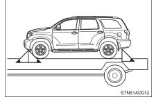
If you use chains or cables to tie down your vehicle, the angles shaded in black must be  $45^{\circ}$ .
