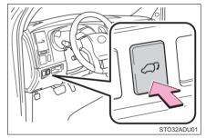
When the switch is pressed again during the halted operation, the back door will perform the reverse operation.
