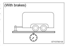
Additional optional equipment, passengers and cargo in the vehicle will reduce the trailer weight rating so as not to exceed GCWR, GVWR and GAWR.
