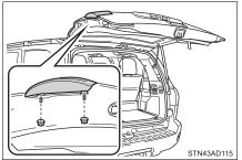
3 Remove the rear combination light assembly in the order shown in the illustration.
