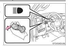
2 Press the Automatic High Beam switch.
