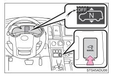
Press the switch again or when the vehicle's speed exceeds 18 mph (30 km/h), the height will be adjusted to the normal height automatically.
