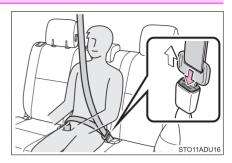
2 To release the hooked plate "A", insert the plate "B" or the key into the hole on the buckle.
