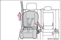
5 If the child restraint has a top tether strap, the top tether strap should be latched onto the top tether strap anchor. (→P. 70)
