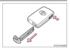
After using the mechanical key, store it in the electronic key. Carry the mechanical key together with the electronic key. If the electronic key battery is depleted or the entry function does not operate properly, you will need the mechanical key.  $(\rightarrow 505)$
