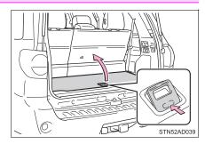
2 Remove the cover and loosen the strap.
