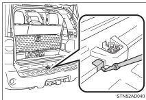
3 Insert the end of the jack handle extension into the lowering screw and turn it counterclockwise.
