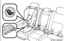
Seat belts equipped with a child restraint locking mechanism (ALR/ELR belts except driver's seat belt) (→P. 34)
