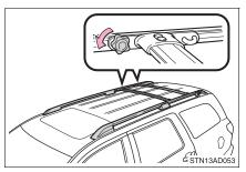
2 Slide the cross rails to the appropriate position for loading luggage and turn the knobs clockwise to tighten the cross rails securely.
