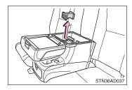
► On the rear console box Pull the separator up.
