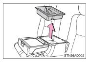
• When closing the rear console box lid, close the rear console box by lifting the grip on the inside of the upper box.
