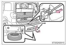
4 Pull out the spare tire and remove the holding bracket.
