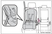
3 Fully extend the shoulder belt and then allow it to retract slightly in order to activate the ALR lock mode.
