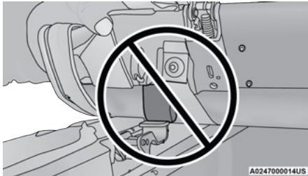
Incorrectly Seated Retainer
