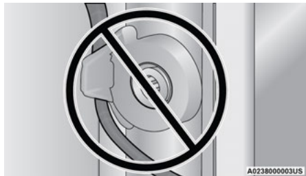
Incorrectly Seated Tailgate Strap
