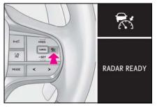
2 Accelerate or decelerate, with accelerator pedal operation, to the desired vehicle speed (at or above approximately 30 mph [50 km/h]) and press the "-SET" switch to set the speed.
