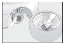
Install the tire and loosely tighten each wheel nut by hand by approximately the same amount. Turn the wheel nuts until the washers come into contact with the disc wheel.
