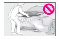
When closing the trunk lid, make sure to press it lightly on its outer surface. If the trunk grip is used to fully close the trunk lid, it may result in hands or arms being caught.
