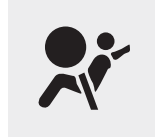
SRS warning light
