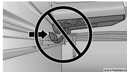
Improper Clamp Position
