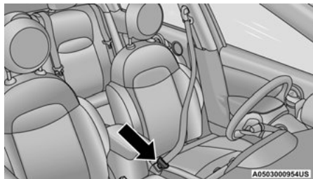
Inserting Latch Plate Into Buckle
