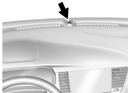
The vehicle has a light sensor on top of the instrument panel. Make sure it is not covered, or the headlamps will be on when they are not needed.
