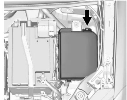
To remove the fuse block cover, squeeze the clip and lift it up.
