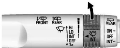
**INT** : Use this setting for intermittent wipes or Rainsense™, if equipped. For intermittent wipes, move the windshield wiper lever to INT. Turn the
