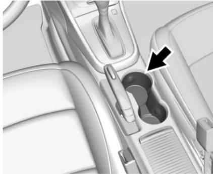
1. Place the transmitter in the center console front cupholder with the buttons facing the front of the vehicle.
