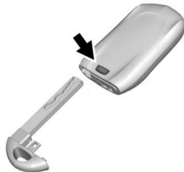
1. Press the button on the back of the RKE transmitter and pull the key out. Never pull the key out without pressing the button.
