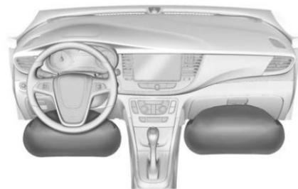
The driver knee airbag (if equipped) is below the steering column. The front outboard passenger knee airbag (if equipped) is below the glove box.
