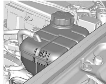
3. Fill the coolant surge tank with the proper mixture to the indicated level mark.
