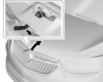
2. Go to the front of the vehicle and locate the secondary release lever under the front center of the hood. Push the secondary hood release lever to the right to release.
