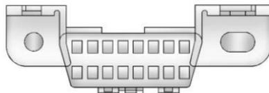
The DLC is under the instrument panel to the left of the steering wheel. Connecting devices that are not used to perform an Emissions Inspection/Maintenance test or to service the vehicle may affect vehicle operation. See *Add-On Electrical Equipment* ⇨ 185. See your dealer if assistance is needed.
