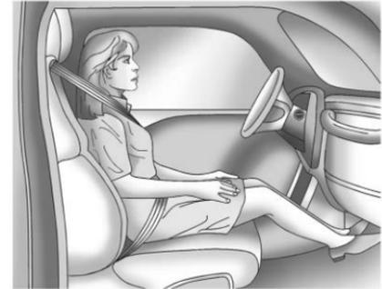
If a person of adult size is sitting in the front outboard passenger seat, but the OFF indicator is lit, it could be because that person is not sitting properly in the seat. Use the following steps to allow the system to detect that person and enable the front outboard passenger frontal airbag and knee airbag (if equipped):
