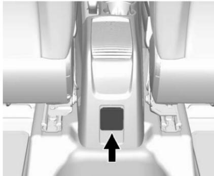
An indicator light on the outlet turns on to show it is in use. The light comes on when the ignition is on and equipment requiring less than 150 watts is plugged into the outlet, and no system fault is detected.
