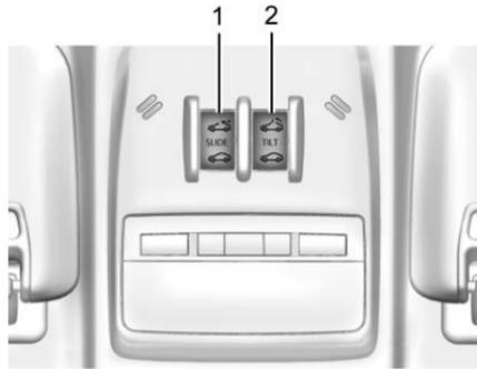
If equipped, the sunroof only operates when the ignition is on or when Retained Accessory Power (RAP) is active. See *Retained Accessory Power (RAP)* ⇨ 156.
