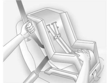
5. To tighten the belt, push down on the child restraint, pull the shoulder portion of the belt to tighten the lap portion of the belt, and feed the shoulder belt back into the retractor. When installing a forward-facing child restraint, it may be helpful to use your knee to push down on the child restraint as you tighten the belt.
