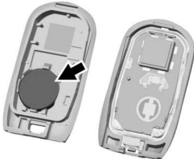
3. Remove the battery by pushing on the battery and sliding it toward the bottom of the transmitter.
