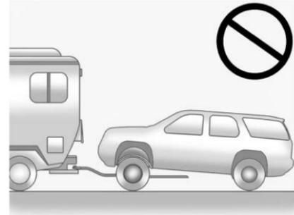
All-wheel-drive vehicles must not be towed with two wheels on the ground. To properly tow these vehicles, they should be placed on a platform trailer with all four wheels off of the ground.
