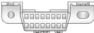
The DLC is under the instrument panel to the left of the steering wheel. Connecting devices that are not used to perform an Emissions Inspection/Maintenance test or to service the vehicle may affect
