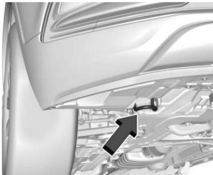
The vehicle is equipped with a specific attachment point to be used by the towing provider. This point may be used to pull the vehicle from a flat road surface onto the flatbed tow truck.
