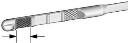
If the oil is below the cross-hatched area at the tip of the dipstick and the engine has been off for at least 15 minutes, add 1 L (1 qt) of the recommended oil and then recheck the level. See “Selecting the Right Engine Oil” later in this section for an explanation of what kind of oil to use. For engine oil crankcase capacity, see *Capacities and Specifications* ⇨ 276.
