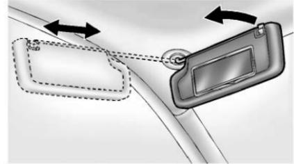
Pull the sun visor down to block glare. If equipped, detach the sun visor from the center mount to pivot to the side window or to extend along the rod.
