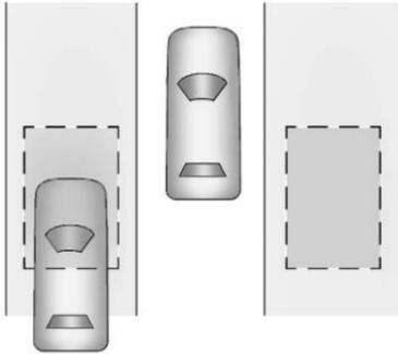
The SBZA sensor covers a zone of approximately one lane over from both sides of the vehicle, or 3.5 m (11 ft). The height of the zone is approximately between 0.5 m (1.5 ft) and 2 m (6 ft) off the ground. This zone starts at approximately the middle of the vehicle and goes back 5 m (16 ft).
