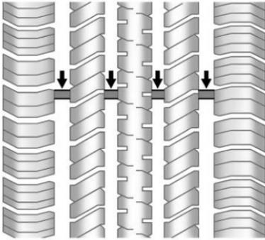
Treadwear indicators are one way to tell when it is time for new tires. Treadwear indicators appear when the tires have only 1.6 mm (1/16 in) or less of tread remaining. See *Tire Inspection* ⇨ 232 and *Tire Rotation* ⇨ 232.
