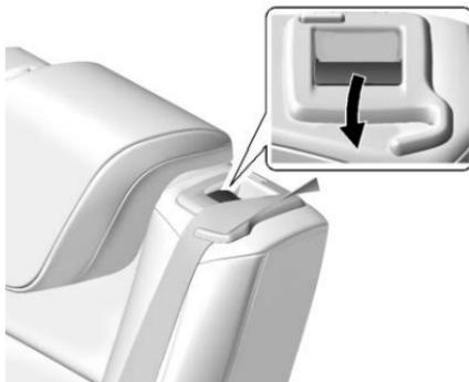
6. Reach under the belt and pull the lever on top of the seatback to unlock the seatback.
