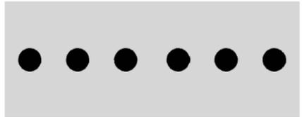
When your vehicle approaches another detected vehicle too rapidly, the FCA display will flash on the windshield. Also, eight rapid high-pitched beeps will sound from the front. When this Collision Alert occurs, the brake system may prepare for driver braking to occur more rapidly which can cause a brief, mild deceleration. Continue to apply the brake pedal as needed. Cruise control may be disengaged when the Collision Alert occurs.
