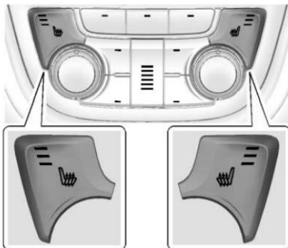
If equipped, the controls are on the climate control panel. The engine must be running to operate the heated seats.
