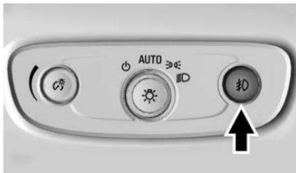
The fog lamps button is on the instrument panel beside the steering wheel.
