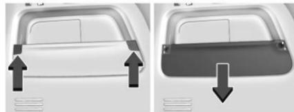
1. Remove the cover and screws attaching the panel to the vehicle interior. Remove the panel.
