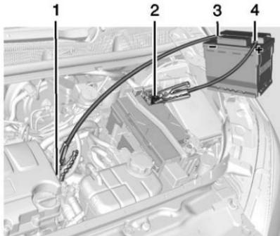
1. Discharged Battery Negative Grounding Point
