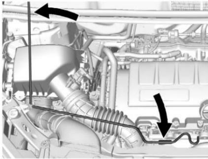
3. Lift the hood and release the hood prop rod from its retainer, in the front of the engine compartment. Securely insert the rod end into the slot marked with an arrow, on the underside of the hood.
