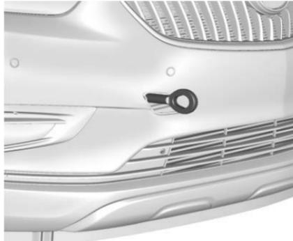
Install the tow eye into the socket by turning it clockwise until it stops. When the tow eye is removed, reinstall the cover with the notch in the original position.
