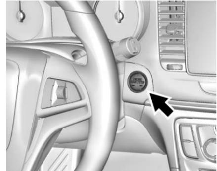
The vehicle has an electronic keyless ignition with pushbutton start. The RKE transmitter must be in the vehicle for the system to operate.
