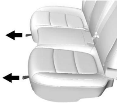
4. Pull the strap on the front edge of the rear seat cushion to release the cushion. Tilt the seat cushion forward toward the front of the vehicle.
