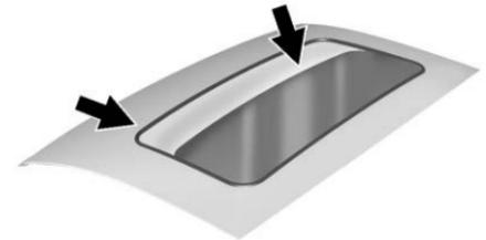
Dirt and debris may collect on the sunroof seal or in the track. This could cause an issue with sunroof operation or noise. It could also plug the water drainage system.
