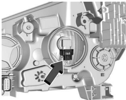
4. Disconnect the wiring harness connector from the bulb.
