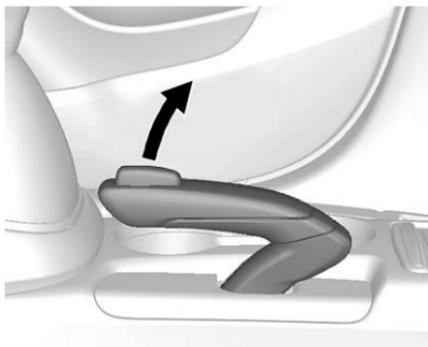
To set the parking brake, hold the brake pedal down and pull up on the parking brake lever. If the ignition is on, the brake system warning light will come on. See *Brake System Warning Light* ⇨ 105.
