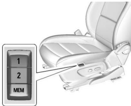
If equipped, the MEM, 1, and 2 buttons on the outboard side of the driver seat are used to manually save and recall the driver seat and outside mirror positions. These manually stored positions are referred to as Button Memory positions.
