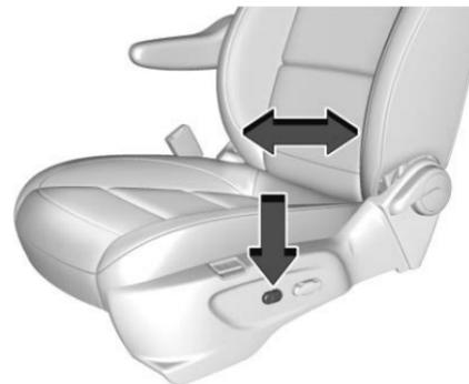
If available, press the front or rear of the switch to increase or decrease lumbar support. Release the switch when the desired level of support is reached.
