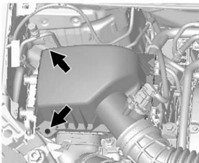
1. Remove the two screws, tilt the cover, and slide it out of the assembly.
