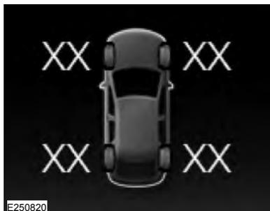
The tire pressure monitoring system measures pressure in your road tires and sends the tire pressure readings to your vehicle. You can view the tire pressure readings through the information display. See **General Information** (page 95). The low tire pressure warning light will turn on if the tire pressure is significantly low. Once
