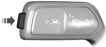
Press the button on the direction indicator stalk to switch the system on or off.
