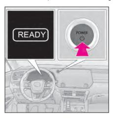
3 Press the power switch shortly and firmly.
