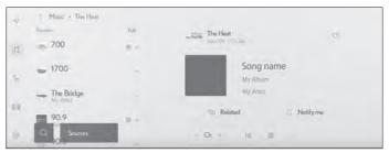
[Ch]: Touch [-] or [+] to search for the receivable channels. Touch and hold to switch channels. When released, the current channel is received.
