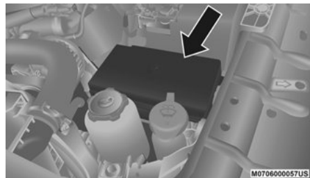
Power Distribution Center Location
