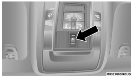
Power Sliding Rear Window Switch
