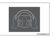
If the driver continues to keep their hands off of the steering wheel, a buzzer sounds and a warning message and the symbol shown in the illustration are displayed on the multi-information display. This warning also operates in the same way when the driver continuously operates the steering wheel only a small amount. Always keep your hands on the steering wheel when using this system, regardless of warnings.
