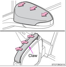
3 Release the claw of the bottom part of the cover and then remove the cover.
