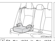
4 Sit the child in the child restraint system. Fit the seat belt to the child restraint system according to the manufacturer's instructions and insert the plate into the buckle. Make sure that the belt is not twisted. High back type
