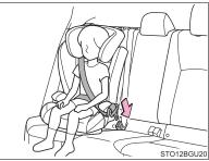
Check that the shoulder belt is correctly positioned over the child's shoulder and that the lap belt is as low as possible. ( $\rightarrow$ P. 26)
