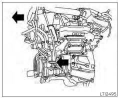
VQ38DD engine **ENGINE SERIAL NUMBER**
