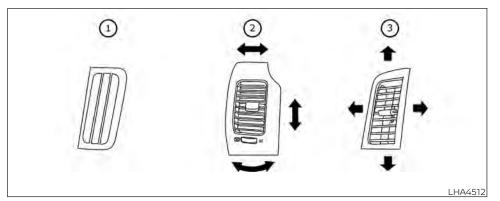
Adjust air flow direction for the vents directed at the driver's and passenger's side windows 1, driver and passenger 2, or center 3 by moving the vent slide and/or vent assemblies. Open or close the driver and passenger vents by using the dial. Move the dial toward the ₹ to open the vents or toward the to close them
