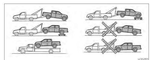
Two-Wheel Drive models with automatic transmission
