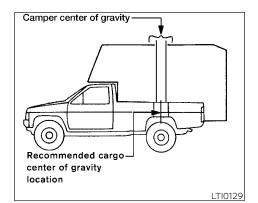
When the truck is used to carry a slide-in camper, the total cargo load of the truck consists of the camper manufacturer's weight figure,
