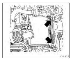
The dry paper type filter element may be cleaned and reused. Replace it according to the maintenance log shown in the "Maintenance and schedules" section of this manual. When replacing the filter, wipe the inside of the air cleaner filter housing and the cover with a damp cloth.
