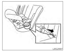
Rear-facing webbing-mounted - step 4 4. Secure the child restraint anchor at-
