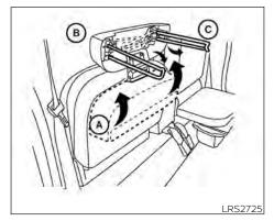
1. To access the jump seat extension (passenger's side only) (A) on the jump seat, pull up (B) on the extension to unfold it to the open position. Then unfold the two support legs (a) and lower the jump seat to the full open seating position.
