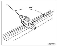
3. Insert the cleat into the channel perpendicular to the channel as shown. Then rotate the cleat clockwise 90° and slide it to the desired location.
