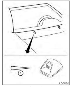
If you wax the surface of the hood, be careful not to let wax get into the windshieldwasher nozzle. This may cause clogging or improper windshield-washer operation. If wax gets into the nozzle, remove it with a needle or small pin (1).
