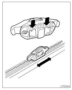
4. Position the cleat so the nubs on the bottom fully seat into the channel detents.
