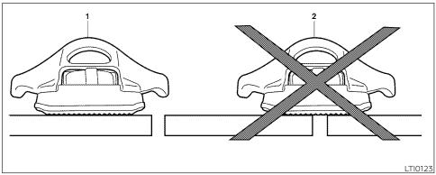
1 correct installation, 2 incorrect installation
