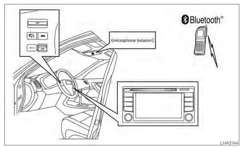
Your NISSAN is equipped with the Bluetooth® Hands-Free Phone System. If you have a compatible Bluetooth® enabled cellular phone, you can set up the wireless connection between your cellular phone and the in-vehicle phone module. With Bluetooth® wireless technology, you can
