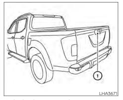
To display the rear view, the Rear View Monitor system uses a camera located next to the tailgate handle  $\bigcirc$ .
