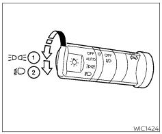
Type A (if so equipped) HEADLIGHT CONTROL SWITCH Lighting
