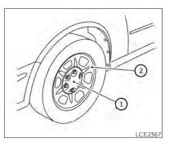
Removing bolt-on wheel caps (if so equipped)
