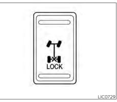
The E-Lock system can help provide added traction if the vehicle is stuck or becoming stuck
